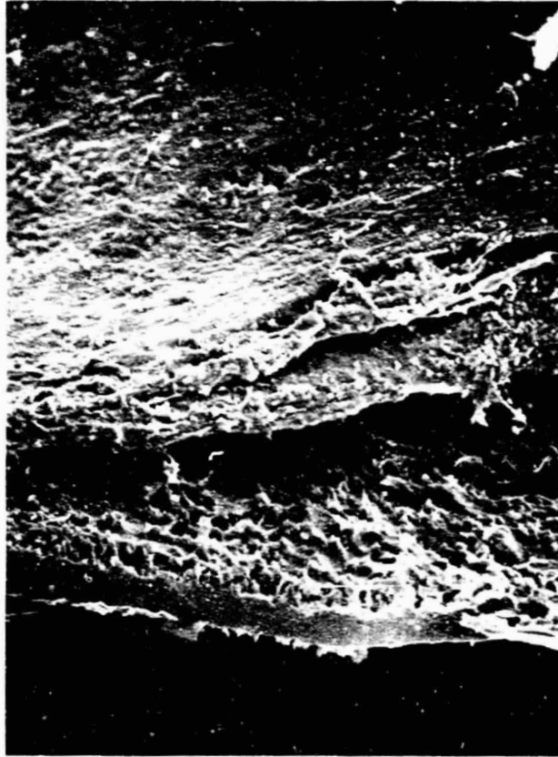
Figure 26. - PTFE NT. Cross section of 14-day implant. There are multiple cell layers, and the natural texture appears to be filled in with an amorphous material.
