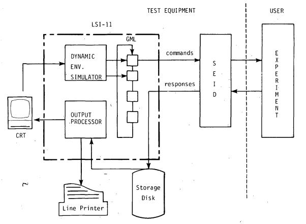
In those situations where even more computer power may be necessary the SEID can be interfaced to a user (or  $I^2$ -) supplied computer. This configuration enables the use of a GML simulation.
