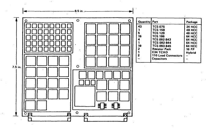
BUILD AND FUNCTIONAL TEST OF PRINTED CIRCUIT BOARDS FOR PROCESSOR MODULE, MEMORY MANAGEMENT UNIT, PRIORITY INTERRUPT CONTROLLER, AND 8K MEMORY MODULE
