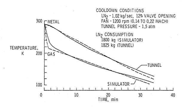
Figure 8. Cool-down profile for tunnel and simulator.
