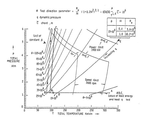
Figure 15. Test direction design in cryogenic wind tunnels—locus of least liquid nitrogen consumption and least q in P-T plane.
