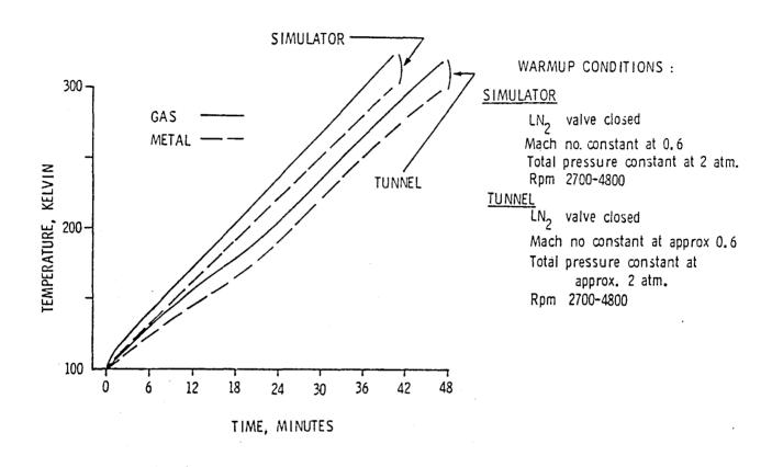
Figure 9. Comparison of tunnel and simulator warmup profiles.
