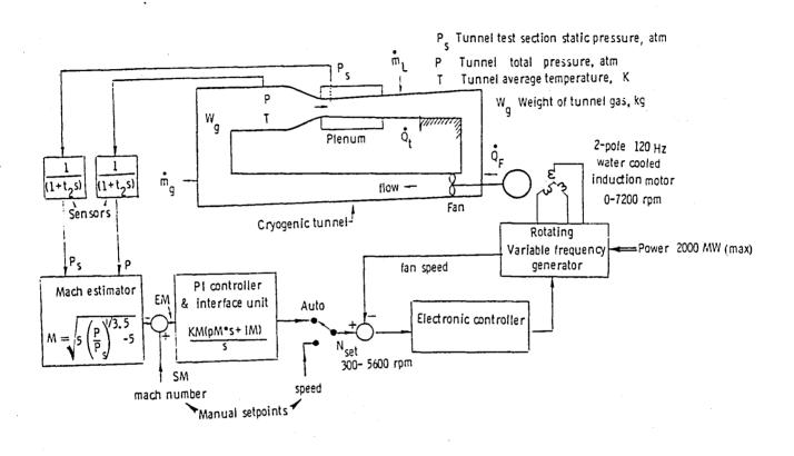
Figure 12. Automatic Mach number control scheme for 0.3-m TCT.
