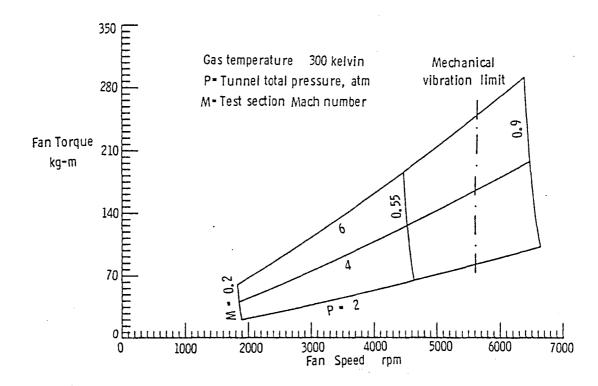
Figure 17. Speed torque characteristics of 0.3-m TCT fan load, 300 K.
