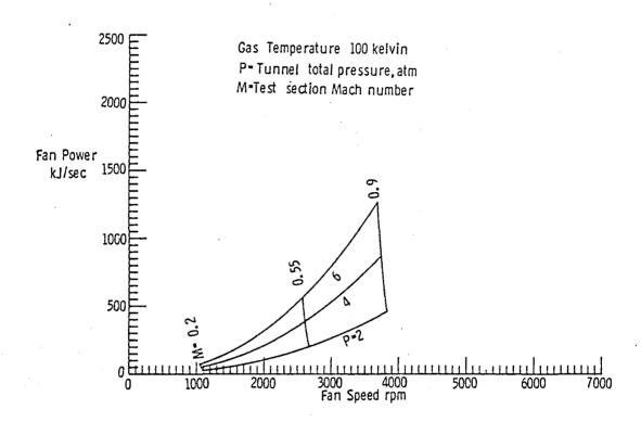
Figure 18. Speed power characteristics of 0.3-m TCT fan load, 100 K.
