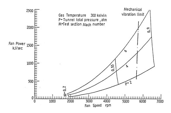
Figure 19. Speed power characteristics of 0.3-m TCT fan load, 300 K.
