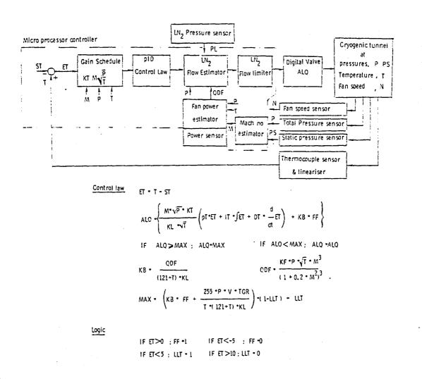
Figure 10. Automatic temperature control scheme for 0.3-m TCT.
