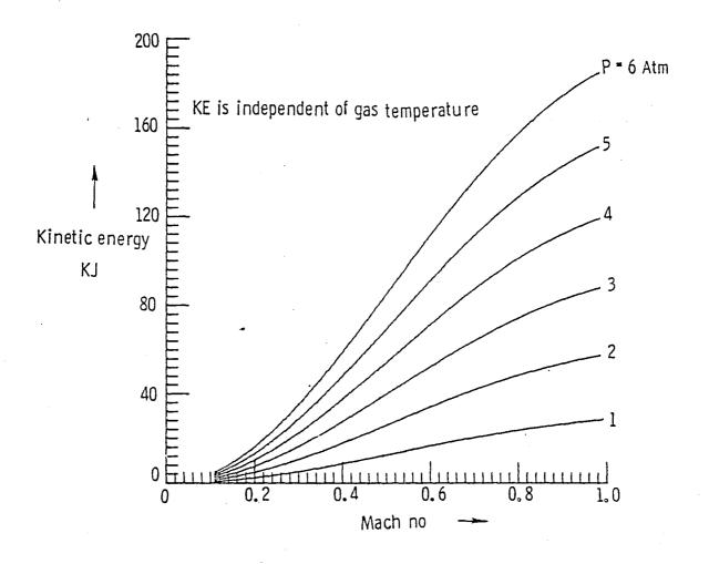
Figure 5. Kinetic energy of nitrogen stream in 0.3-m TCT.
