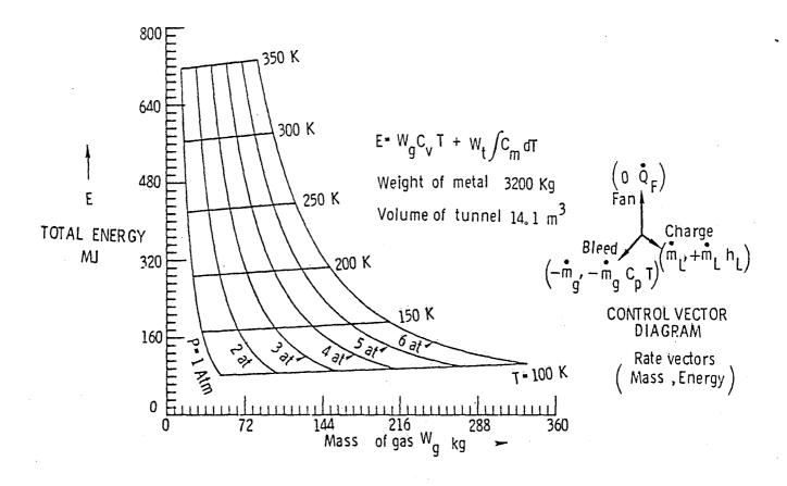
Figure 4. Energy state diagram of gas, 0.3-m TCT.
