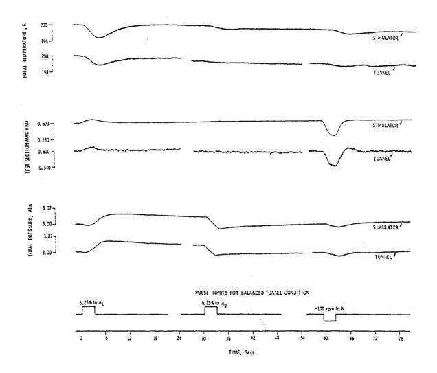
Figure 7. Simulator and tunnel transient response data at T = 200 K, M = 0.6, and P = 3 atm.
