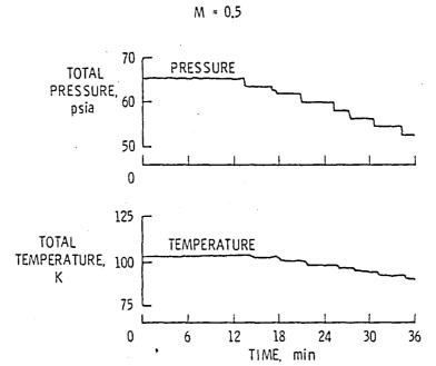
Figure 14. Typical 0.3-m TCT test temperature and pressure on automatic control.
