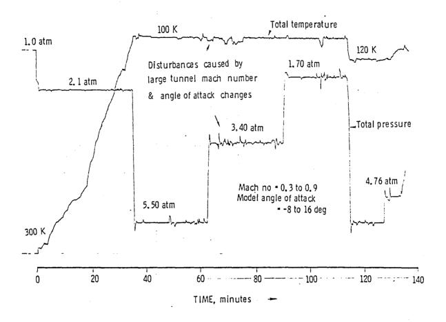
Figure 13. Typical 0.3-m TCT test with temperature and pressure on automatic control.
