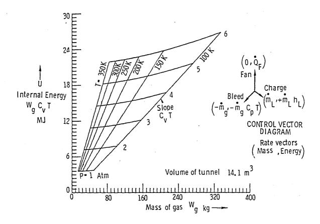
Figure 3. Energy state diagram including metal enthalpy of 0.3-m TCT.
