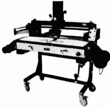
Figure 3.8 Light table and zoom stereoscope. Richards MIM 4 table with motorized film advance and Bausch and Lomb Model 240 stereoscope. (Courtesy The Richards Corporation.)
