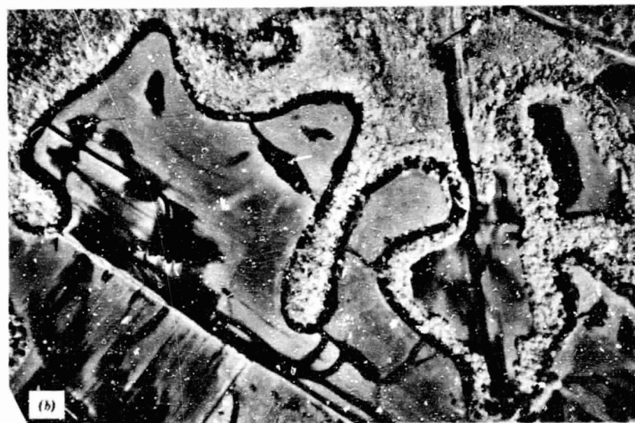
Figure 3.28 Flooding of Bear Creek, northwest Alabama, April 3, 1969, 1:90000. (a) Panchromatic film with a Wratten #12 (yellow) filter, 9:43 A.M. (b) Black and white infrared film with a Wratten #12 filter, 12:51 P.M. (Courtesy Mapping Services Branch, Tennessee Valley Authority )
