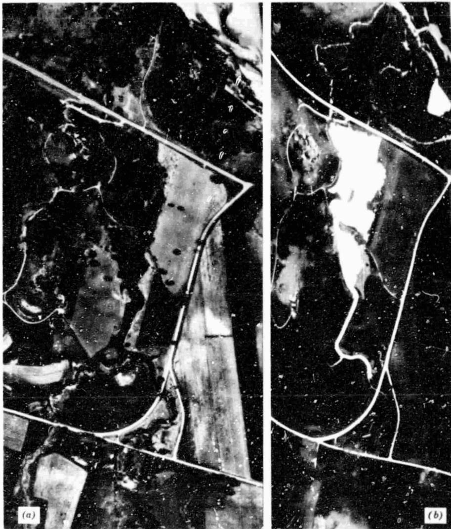
Figure 7.24 Comparison of aerial photograph and thermal image illustrating tangential distortion, Iowa County, Wisconsin. (a) Panchromatic aerial photograph, May 19, 1968, 3000 m flying height. (b) Nonrectified thermal image, 6.00 A.M., September 1971, 300 m flying height. (Aerial photograph courtesy USDA-ASCS; Thermal image courtesy National Center for Atmospheric Research.)
