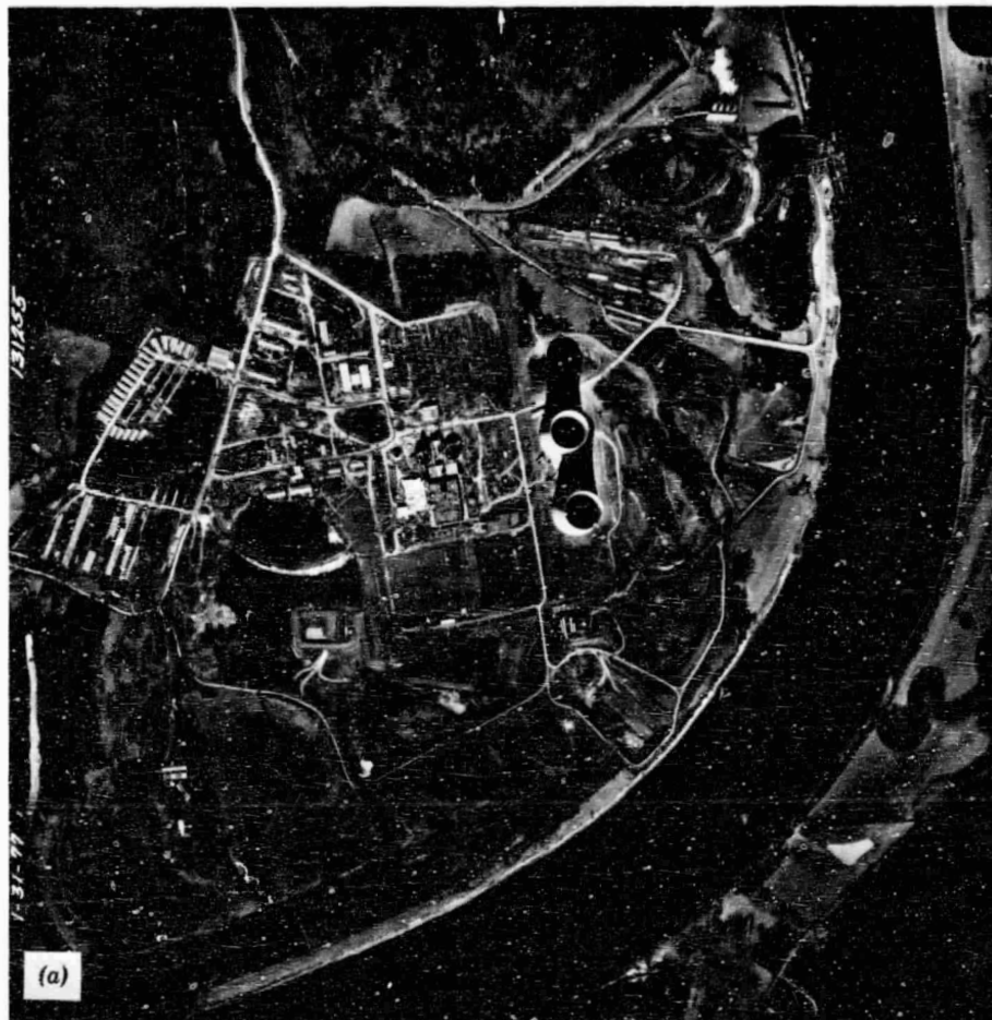
Figure 5.7 Vertical photographs of the Watts Bar Nuclear Power Plant Site, near Kingston, Tennessee, January 31, 1977. In (a) the two plant cooling towers appear near the principal point and exhibit only slight relief displacement. The towers manifest severe relief displacement in (b). (Courtesy Mapping Services Branch, Tennessee Valley Authority.)
