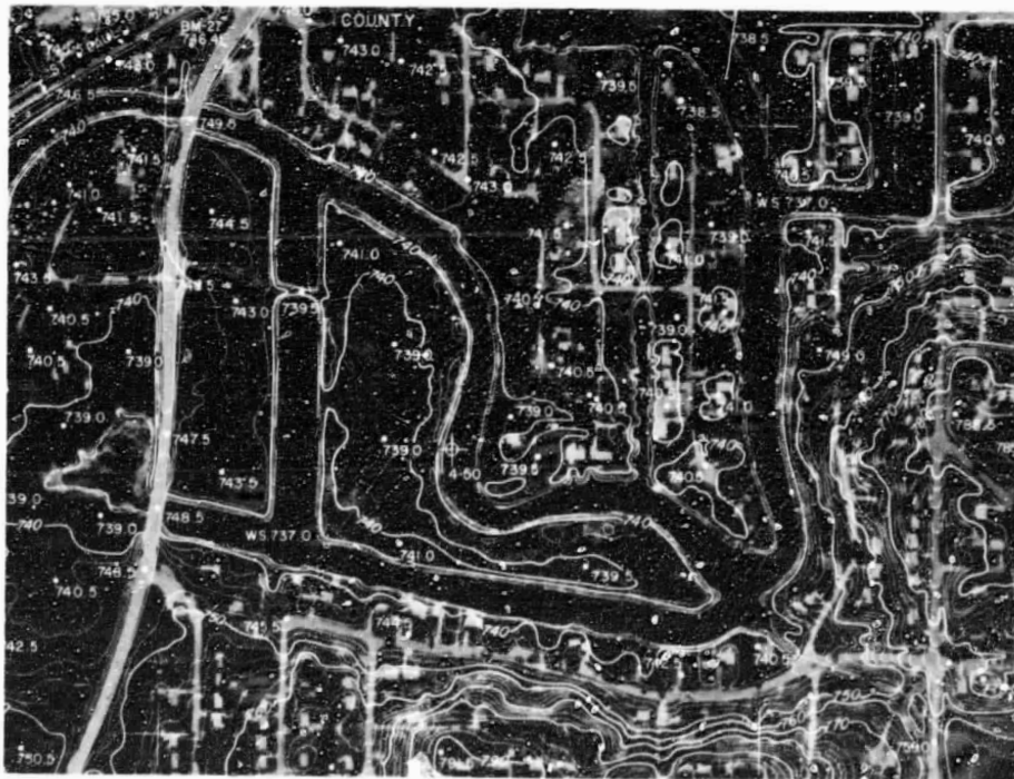
Figure 5.25 Portion of a 1:4800 topographic orthophotomap. Photography taken in 1975 at the Fox Chain of Lakes, Illinois. (Courtesy Alster and Associates, Inc.)
