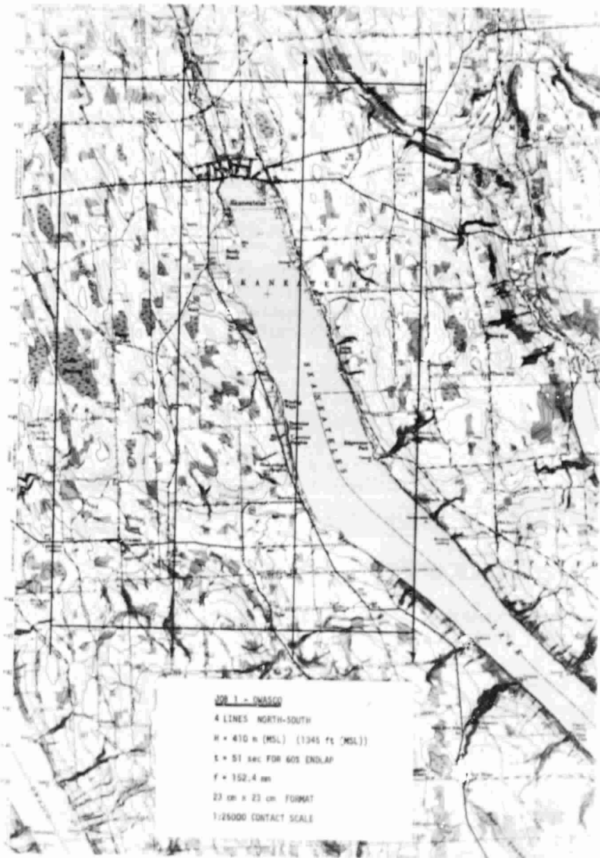
Figure 5.29 Flight map for Example 5.14. (Lines indicate centers of each flight line to be followed.)
