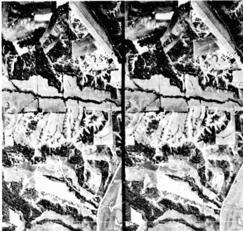
Figure 4.42 Loess in a humid climate. Pottawattamie County, Iowa, September 1966. 1:22,200. (USDA-ASCS photos. Stereogram.)
