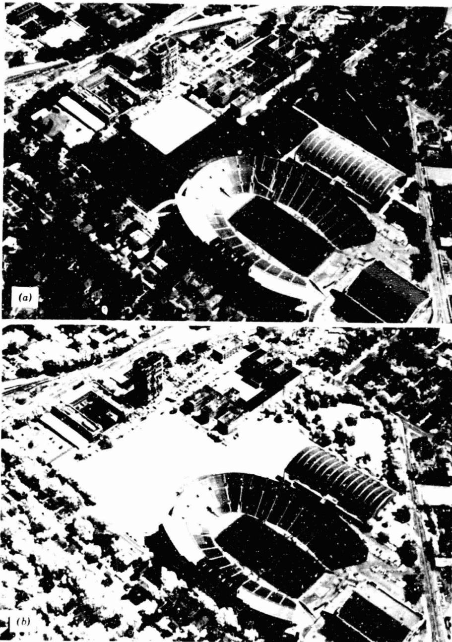
Figure 2.16 Simultaneous oblique aerial photographs showing the effect of filtration on discrimination of ground objects. On panchromatic film (a) natural grass and artificial turf have a similar tone. When scene energy is filtered such that only wavelengths longer than 0.7 \mu\text{m} are incident on black and white infrared film (b) , the natural grass has a very light tone and the artificial turf a very dark tone.
