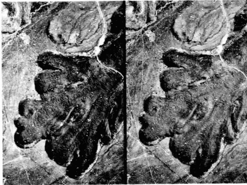
Figure 4.25 Viscous lava flow in an arid climate. Siskiyou County, California, August 1955. 1:33,300. (USDA-ASCS photos. Stereogram.)
