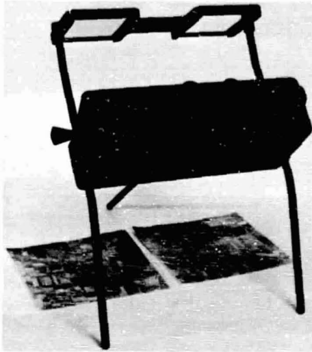
Figure 3.6 Scanning mirror stereoscope. Old Delft Scanning Stereoscope.
