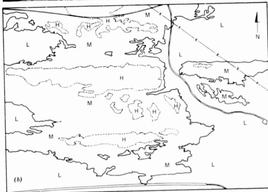
Figure 6.16 Defoliation map obtained by density slicing the photograph shown in Figure 6.14. (a) Density sliced display. (b) Resulting map. Three classes of defoliation severity are shown: high (H), medium (M), and low (L).
