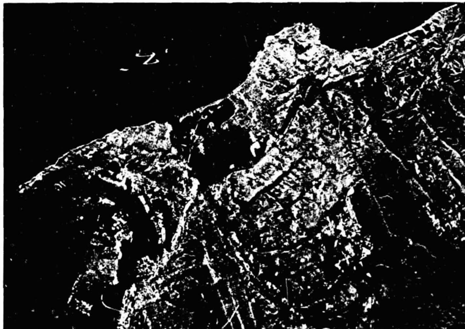
Figure 9.1 SLAR image, San Diego, California. 12,000 m flying height, 1:250,000, X Band, synthetic aperture. (Courtesy Aero Service Division, Western Geophysical Company of America, and Goodyear Aerospace Corp.)
