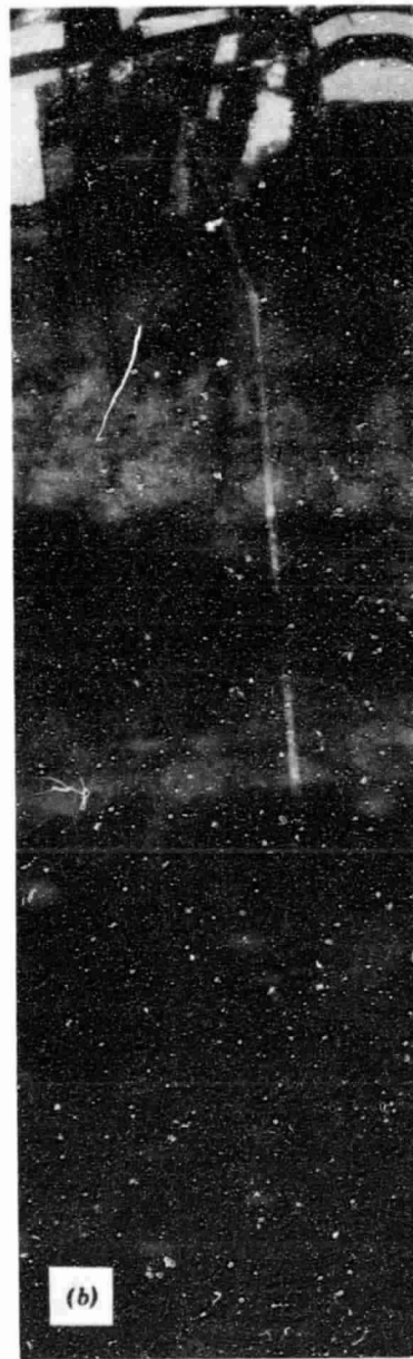
Figure 5.22 Portion of a perspective photograph ( a ) and an orthophoto ( b ) showing a power line clearing traversing hilly terrain. (Note the excessive crookedness of the power line clearing in the perspective photo that is eliminated in the orthophoto). (Courtesy U.S. Geological Survey.)
