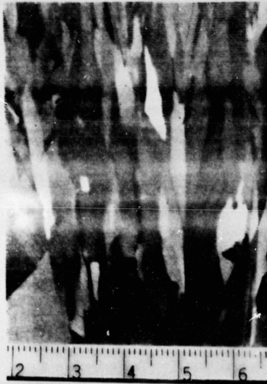
Figure 7. Photograph of Grain Structure in Bridgman-Solidified Silicon Ingot (Scale in mm).
