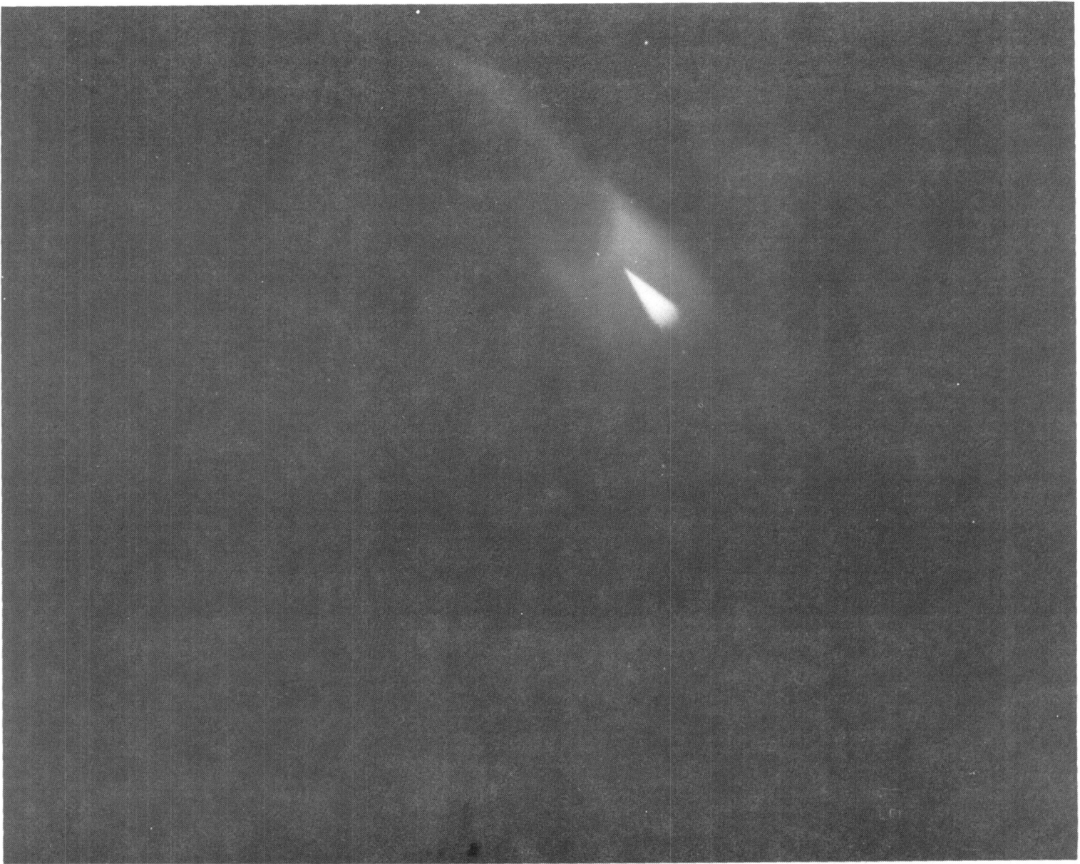
Figure A-4. Exposure from Pt. Barrow, Alaska at time of fourth Cameo barium release. Showing (from left to right) field aligned ion clouds from second and third release, spherically expanding neutral clouds, and the plume of the fourth release.
