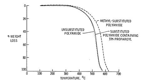
TGA's COMPARING THERMAL STABILITIES OF SUBSTITUTED POLYAMIDES
