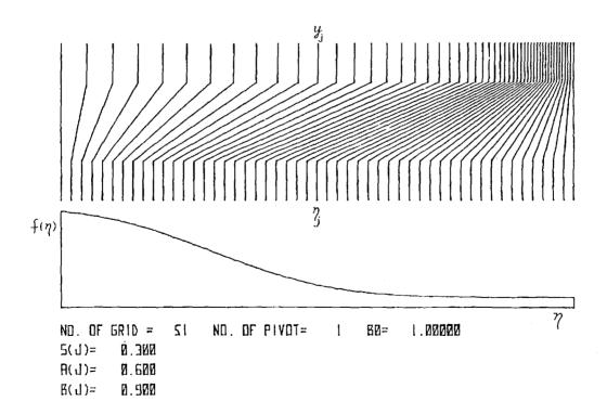
Grids are clustered only at an interior point with a pair of pivots. Specified Parameters
