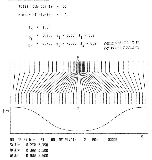
Figure demonstrates smooth variation of grid sizes (large  $|\alpha|$  compare to pivot spacing) with multi-pivots.
