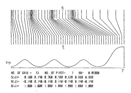
Figure demonstrates discontinuous variation of grid sizes (small  $|\alpha|$  compare to pivot spacing) with multi-pivots.
