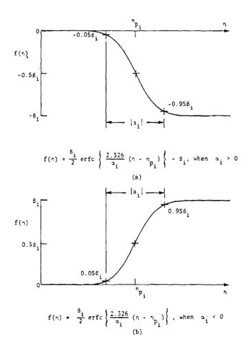
Grids are clustered only at  $\ensuremath{n_{\mbox{min}}}$  with a single pivot.
