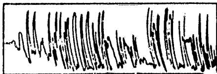
Figure 170 Recording of Vertical Acceleration Caused by A Pigeon Flapping its Wings during Takeoff
