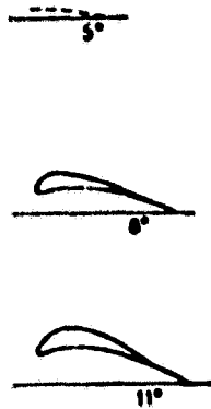
Figure 227 Bearded Vulture Wing with Cross Sections Showing Various Curvatures and Angles of Incidence
