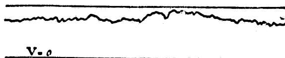
Figure 57 Speed of a WSW Sea Breeze Recorded at the Ile de Ré with a Hot Wire Anemometer 2 M above the Ground 1 sec = 3.5 mm Scale of Speed: 1.3 mm per m/sec
