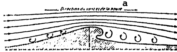
Figure 96 Path of Lower Layers of an Air Current Encountering a Wave
