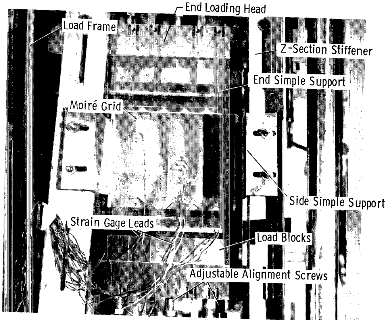
Figure 6.- Buckling specimen in test fixture.
