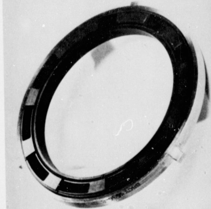
Figure 3. - Face seal with self-acting geometry.
