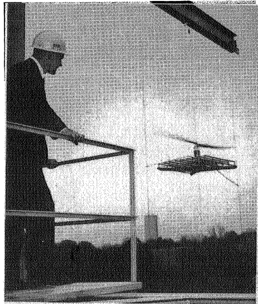
Figure 5. Microwave powered helicopter in flight 18.28 meters above a transmitting antenna. The receiving array for collecting the microwave power and converting it to DC power was made up of several thousand point contact silicon diodes. DC power level was approximately 200 watts. The date of the demonstration was October 1964.
