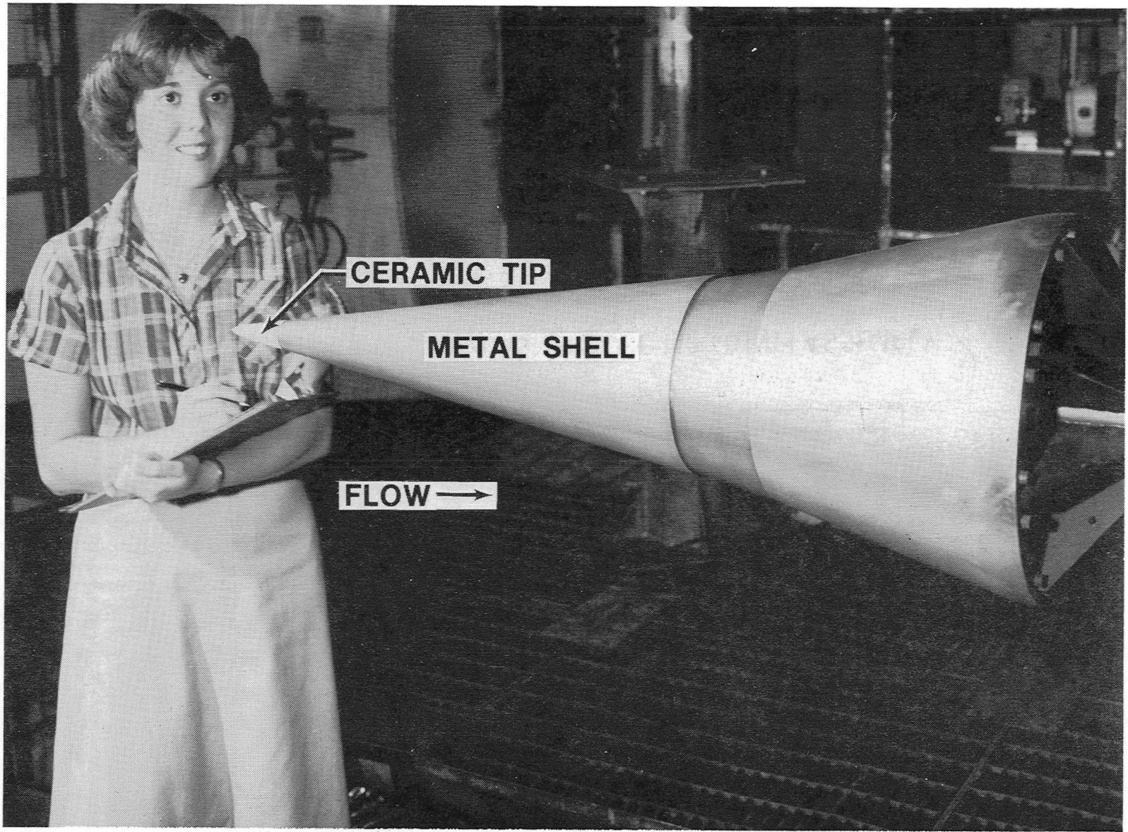
Figure 9.- Photograph of GJNT model in test section of the 8-Ft. HTST.
