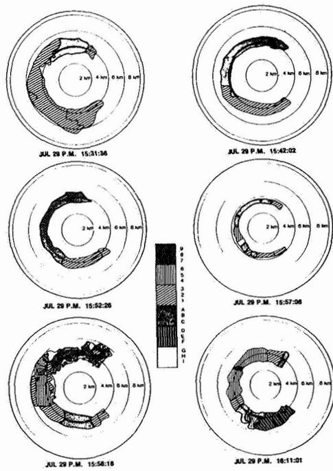
Figure 6.- Wind flow-field plots. Lidar data, July 29, 1978.
