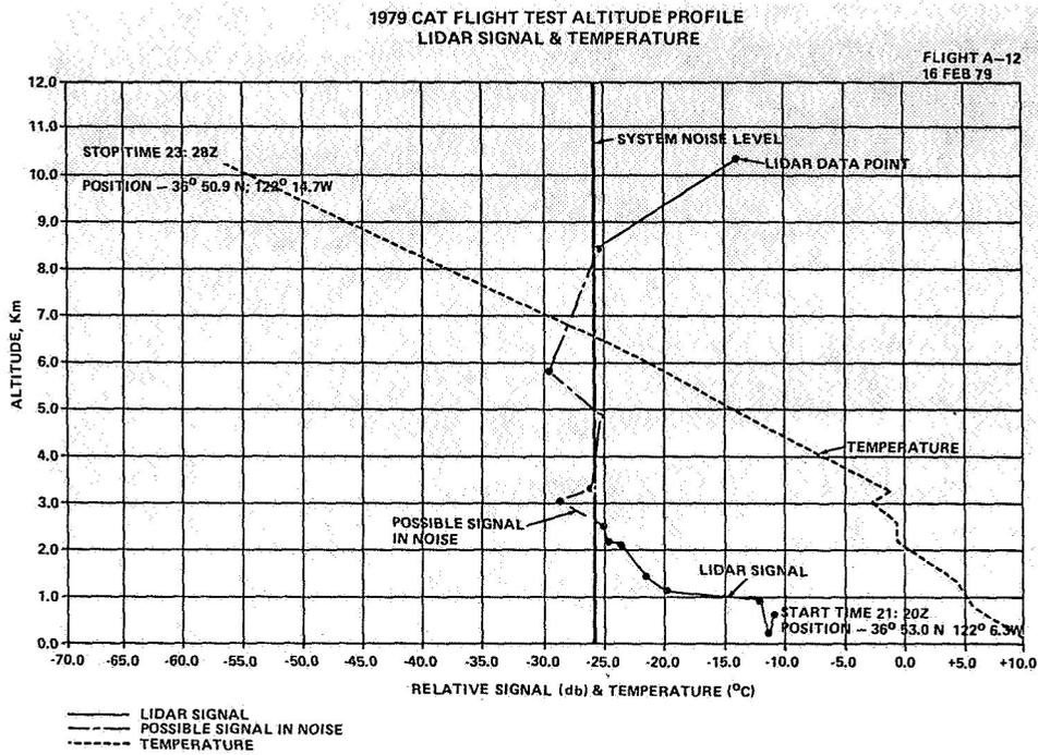
Figure 9.- Lidar signal level variation with altitude.
