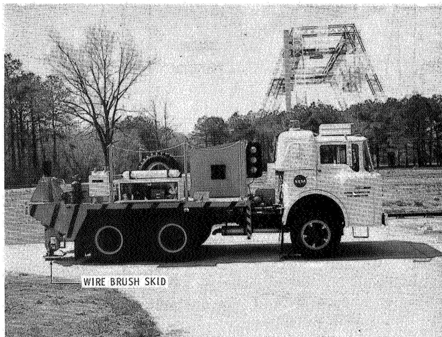
Figure 8.- Instrumented ground vehicle as used for wire brush skid tests.
