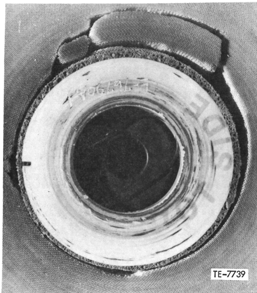
Figure 91. Regenerator disk hub failure encountered during hot rig running.
