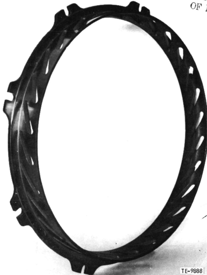
Figure 77. Finish-machined vane outer support ring.
