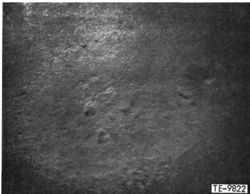
Figure 37. Pure Carbon RB SiC sample II-3 erosion--45° impingement, 0.377 g/min dust flow. (5X)
