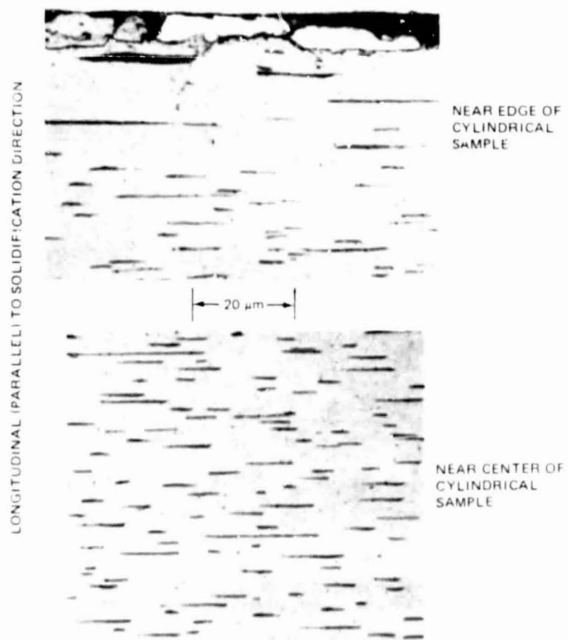
Fig. 15 SPAR VI Flight Sample No. 1 Morphology in Low \bar{g} Interval Longitudinal (Parallel) to Solidification Direction
