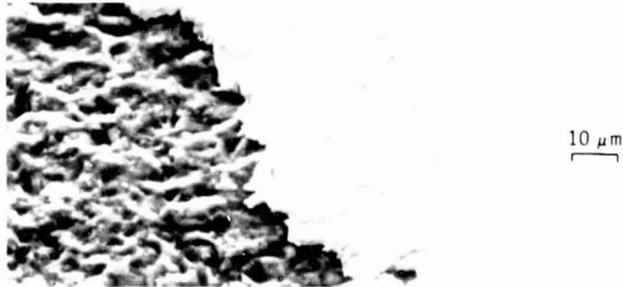
Figure 12 Scanning Electron Microscope View of Aluminum Oxide Surface (Darker Area at Left) and Platinum Film Surface on Blade No. 1 Before Combustor Tests - Adherence of platinum and platinum-10% rhodium films was generally good. The aluminum oxide structure is similar to that of Blade A, Figure 9, previously identified as a "good adherence" surface.
