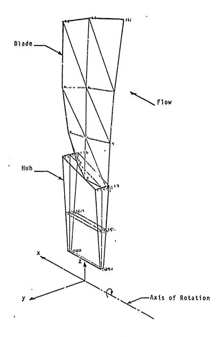
Figure 1. Finite Element Model of an Axial Flow Compressor Rotor Sector, and the Basic Coordinate System
