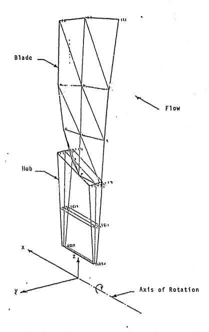
Figure 1. Finite Element Model of an Axial Flow Compressor Rotor Sector, and the Basic Coordinate System
