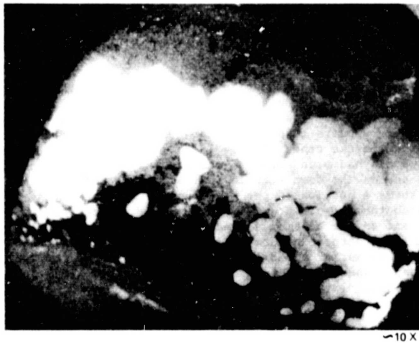
Figure 20. Crystals on Top Surface of "Loaf" Casting
