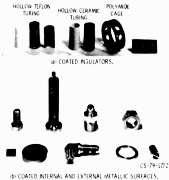
Figure 10. - Ion plated insulators and objects with metallic coating.
