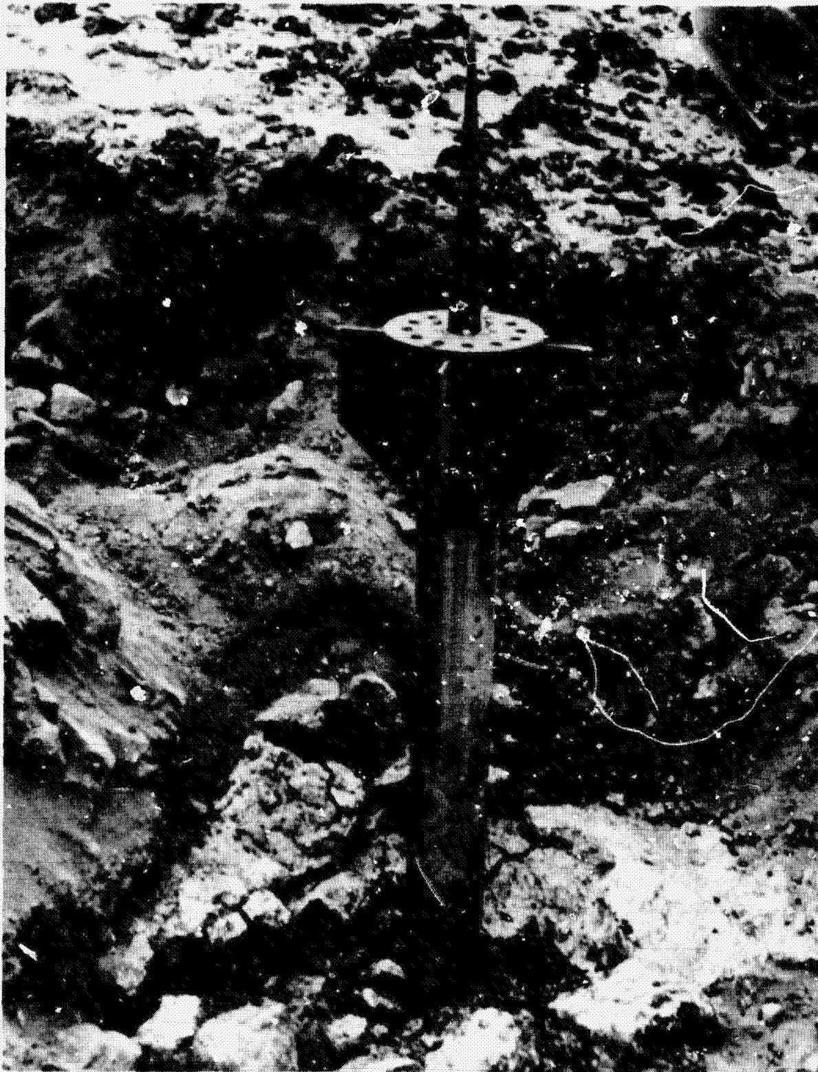
Figure 7.- Radial fractures were produced by the penetrator during emplacement in the basalt; they were revealed when the alluvial overburden was removed.
