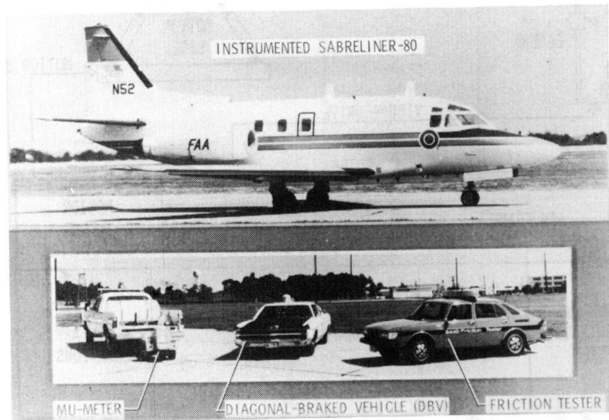
Figure 6.- Test aircraft and ground friction measuring vehicles used in joint NASA/FAA program.
