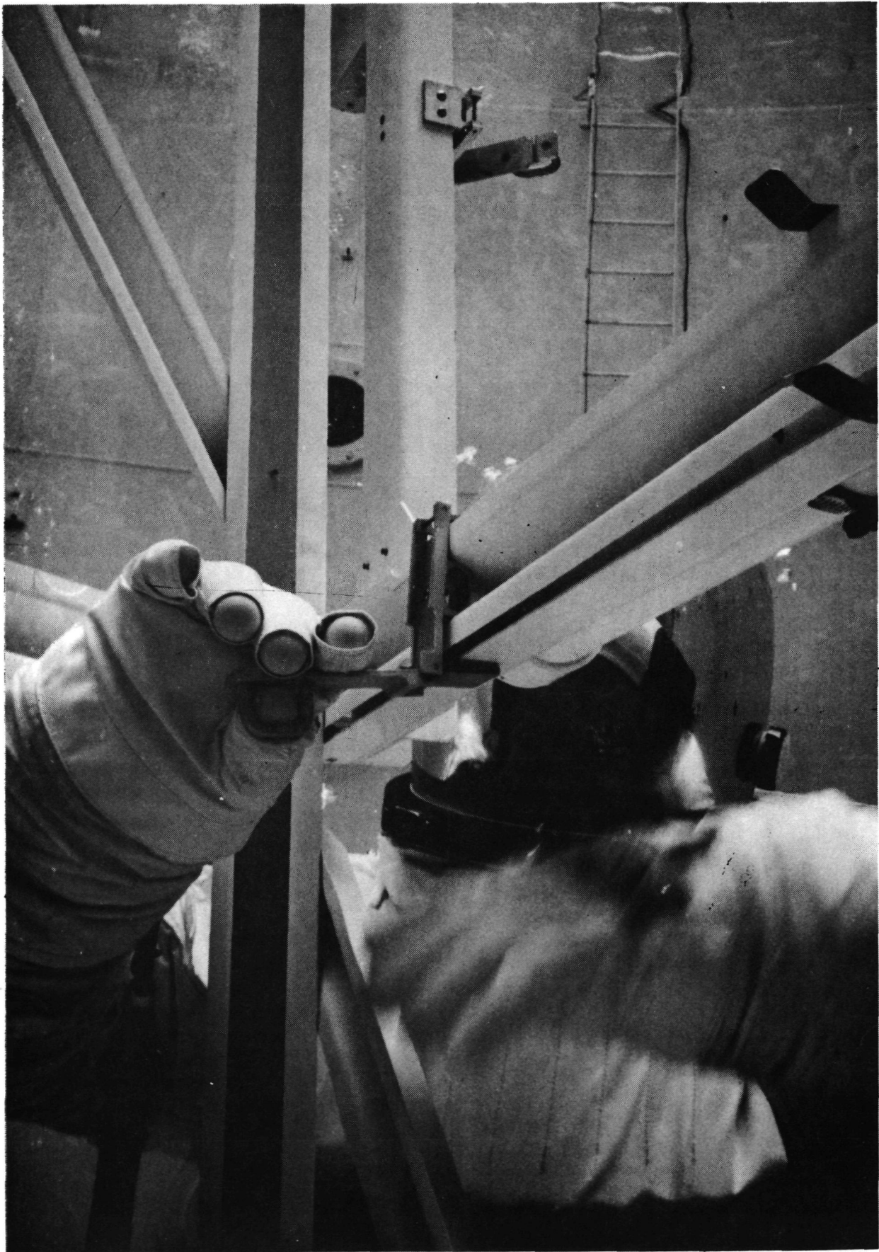
Figure 3-5: Lap Joint During Test
