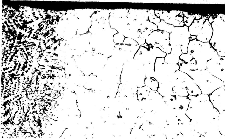
B. - Cross Section at Weld Interface: Cast Dendritic Structure of Weld at Left and Base Material Grain Structure at Right Mag. 100X
