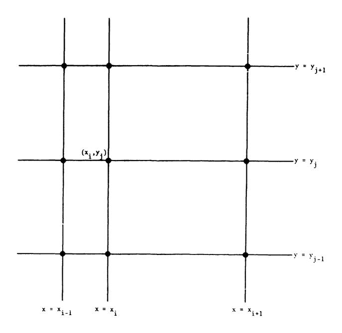
Figure 1. Portion of the grid G which divides the region R into  $(N-1) \times (M-1)$  rectangles. In this sample grid, the spacing is non-uniform in the x-direction and uniform in the y-direction with  $y_{j+1} = y_j + \Delta y$  where  $\Delta y = (d-c)/(M-1)$ .
