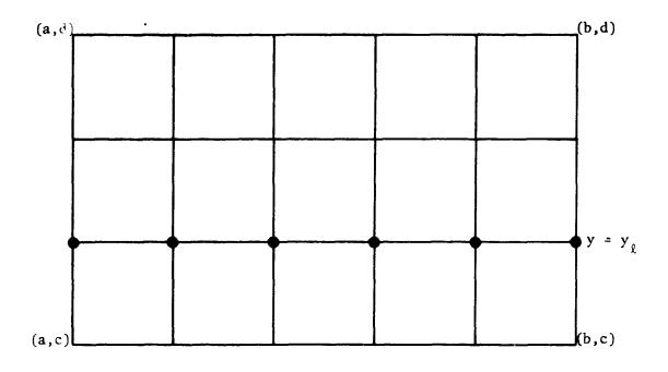
Figure 2. A grid G with N = 6 and M = 4. Grid points marked with lacktriangle denote points at which data is required for computation of the x-integrals  $F_k(y_{\varrho})$  (k = 1, ..., 6) using the integrating matrix [I] based on the grid  $G_{\chi}$ .
