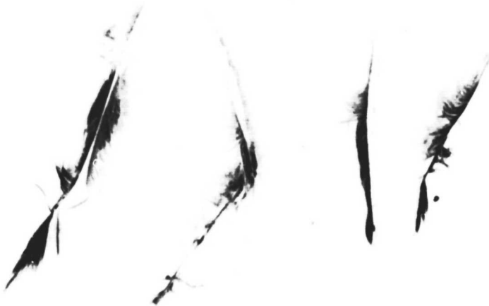
Figure 100 Bird Feathers Taken from the Second-Stage Low-Pressure Compressor Stator Assembly. (ip-444-0374-F)
