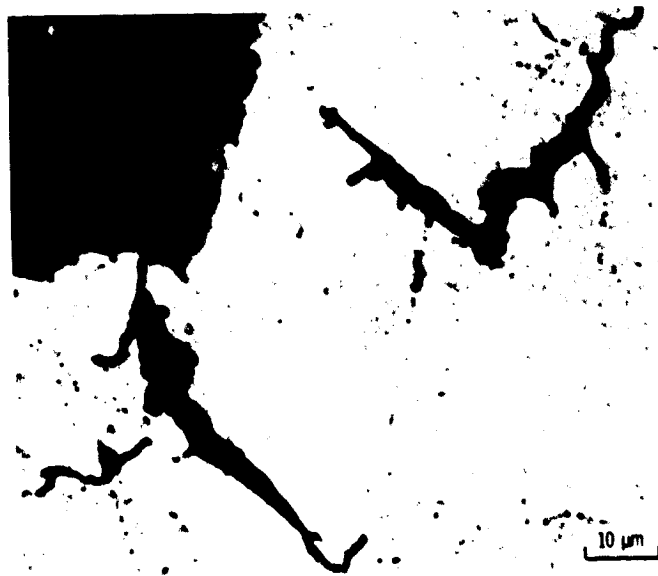
(b) SUBSURFACE CRACKING.
