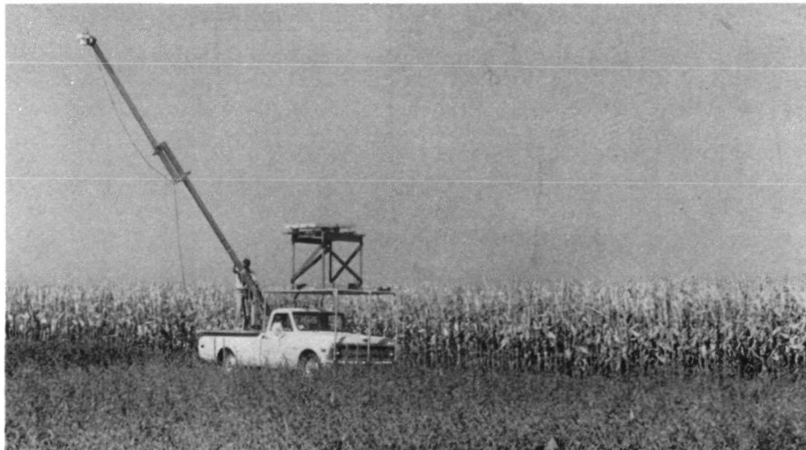
Figure 7. Photograph of truck-mounted boom with multiband radiometer viewing soybean plot.
