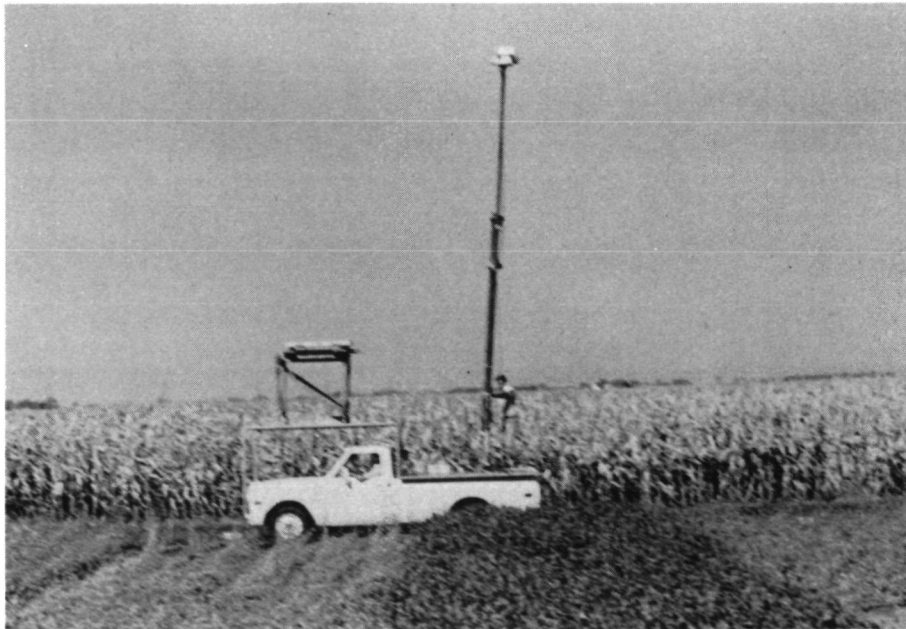
Figure 6. Truck-mounted boom positioning the multiband radiometer.
