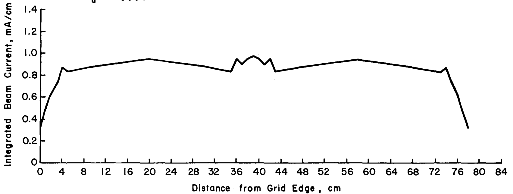
Fig. 5-15. Integrated beam current profile for the best overlap position at 6 \times 10^{-4} Torr and R = 0.50 .
