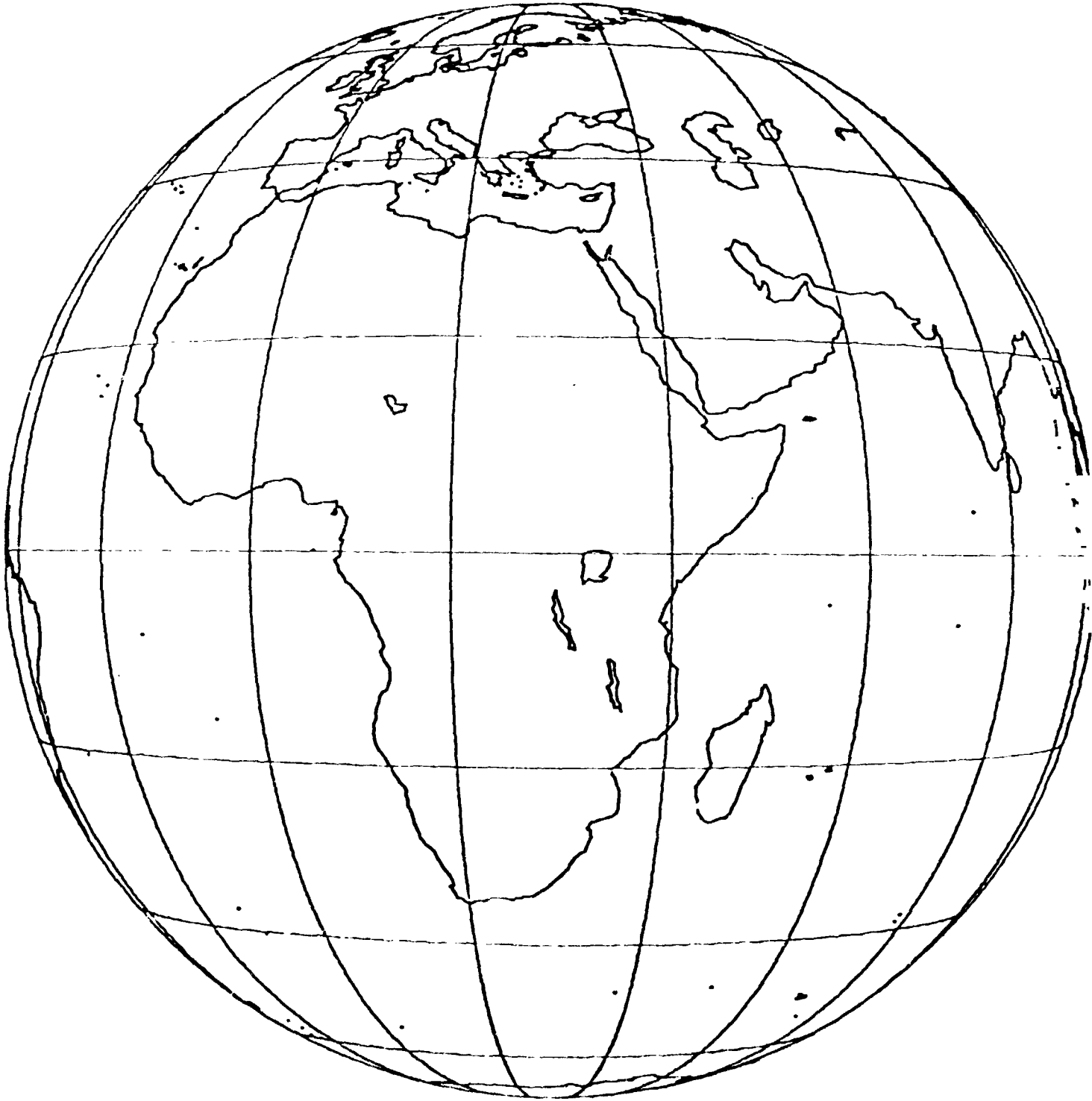
Figure 6. A global perspective view at 29° E from geostationary orbit. A global sensor placed at 29° E longitude would see this view of the world.
