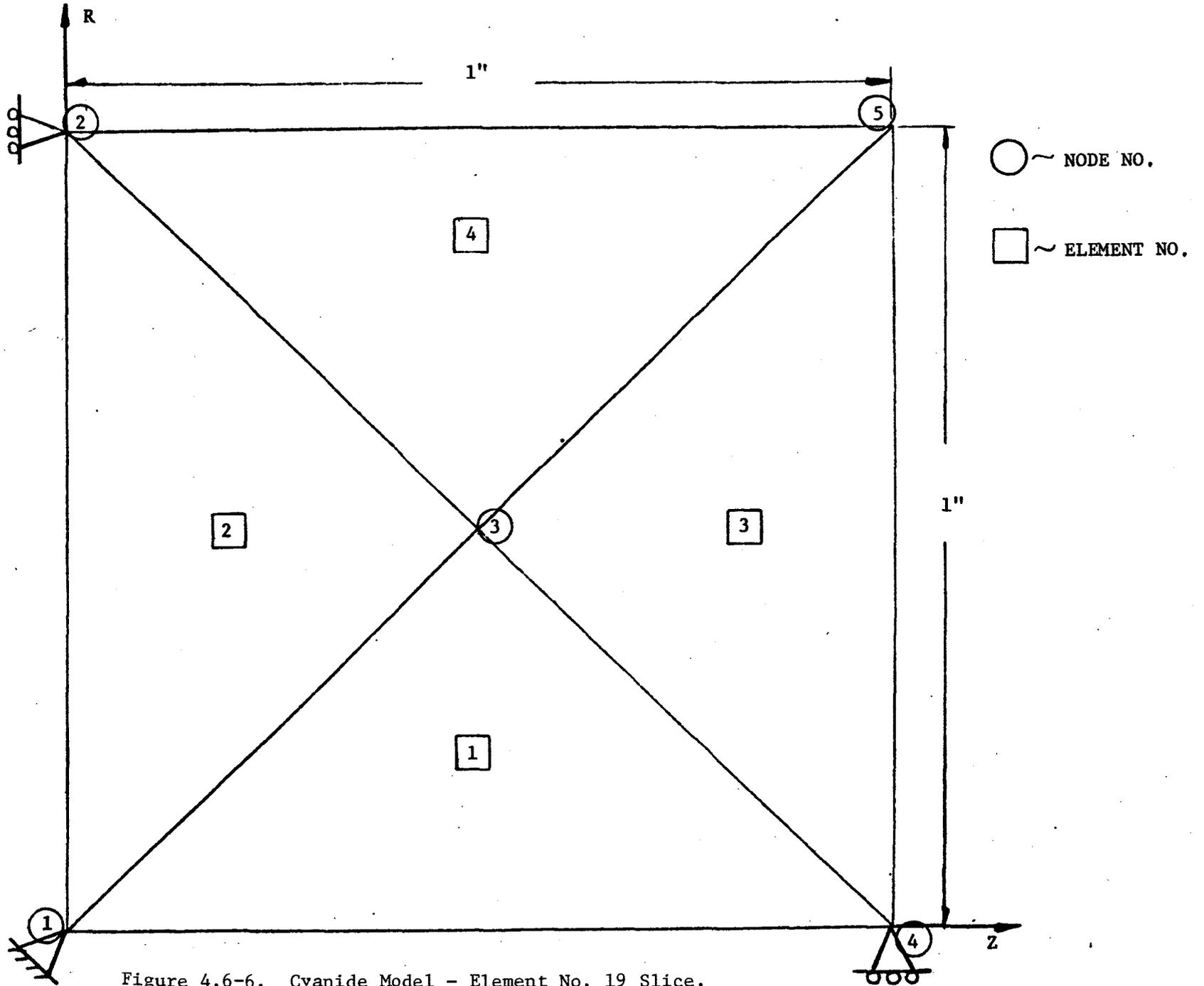
Figure 4.6-6. Cyanide Model - Element No. 19 Slice.
