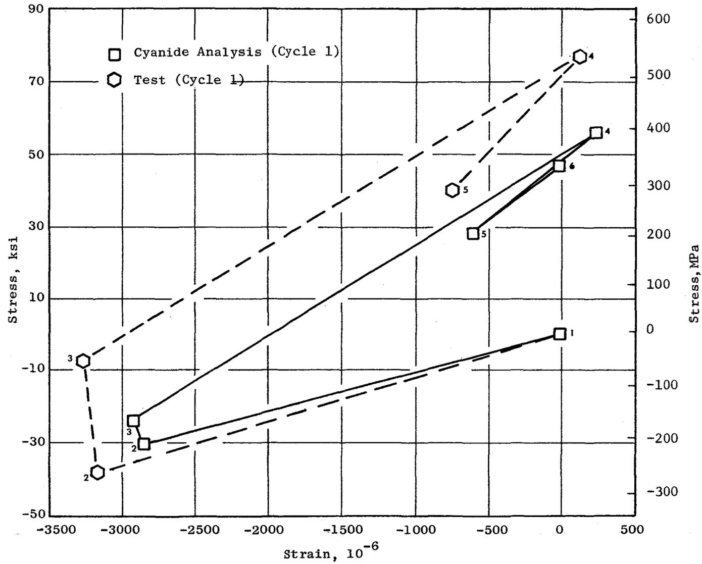
Figure 4.6-17. Stress Versus Strain - Elastic Analysis Profile.
