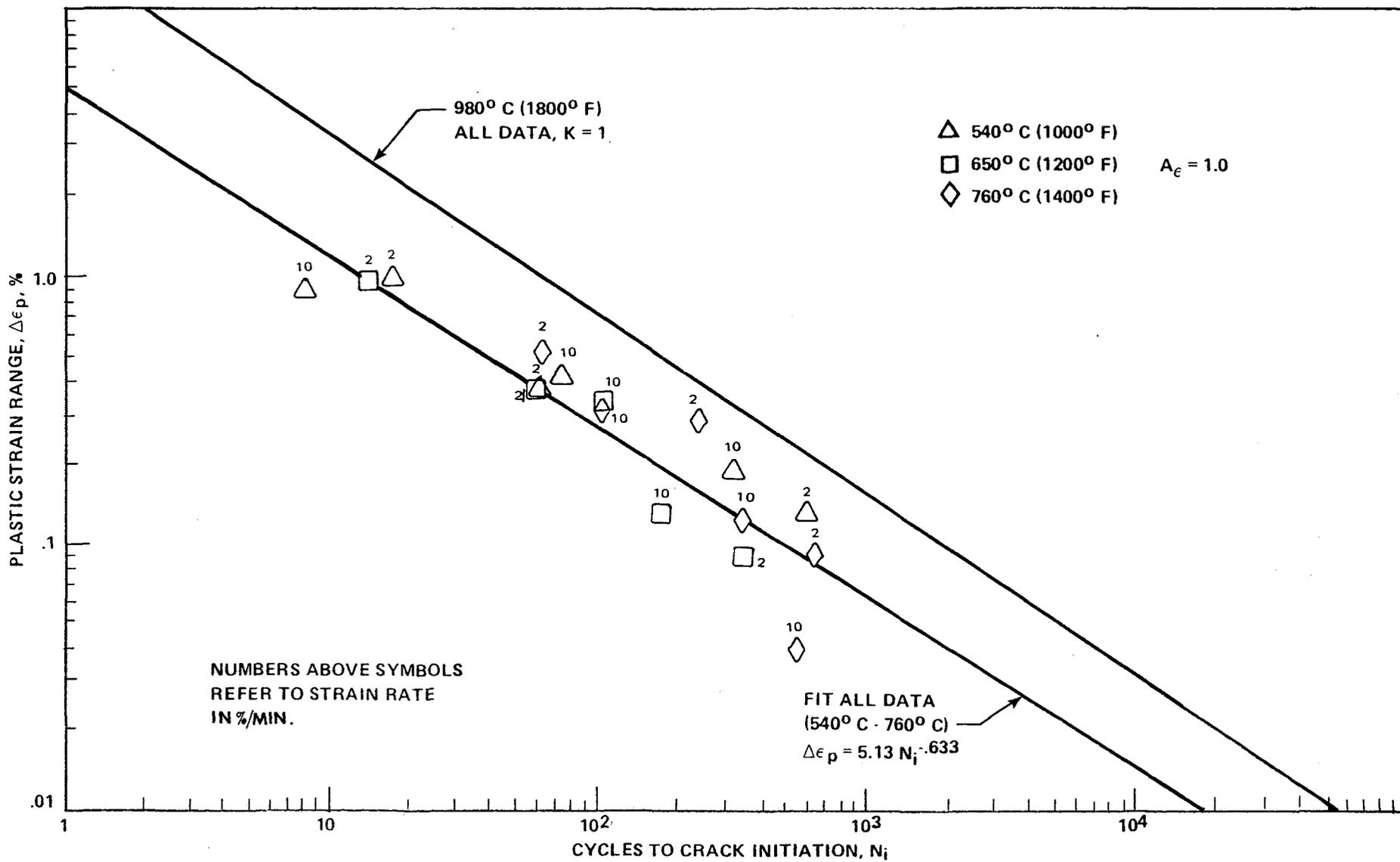
Figure 5.3-7. Plastic Strain Characteristics at Lower Temperatures - René 80.
