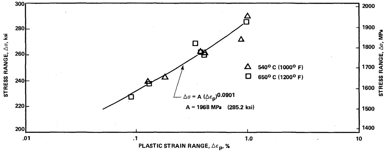
Figure 5.3-8. Fit of  $\Delta\sigma$  vs.  $\Delta\epsilon_p$  at Low Temperatures - René 80.
