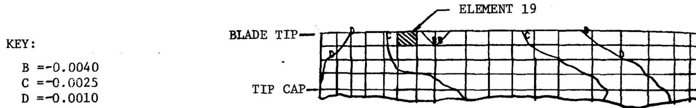
Figure 4.6-3. Blade Tip Model - Contour Plot of Principal Strains - Suction-Side Face.
