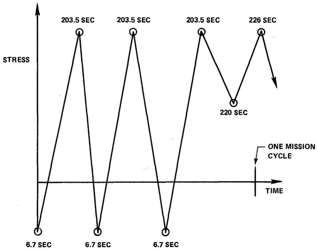
Figure 5.3-14. Schematic of the Assumed Mission Cycles for the Crack Growth Analyses. Times Shown Refer to Analyses Times in Previous Figures and in the Text.
