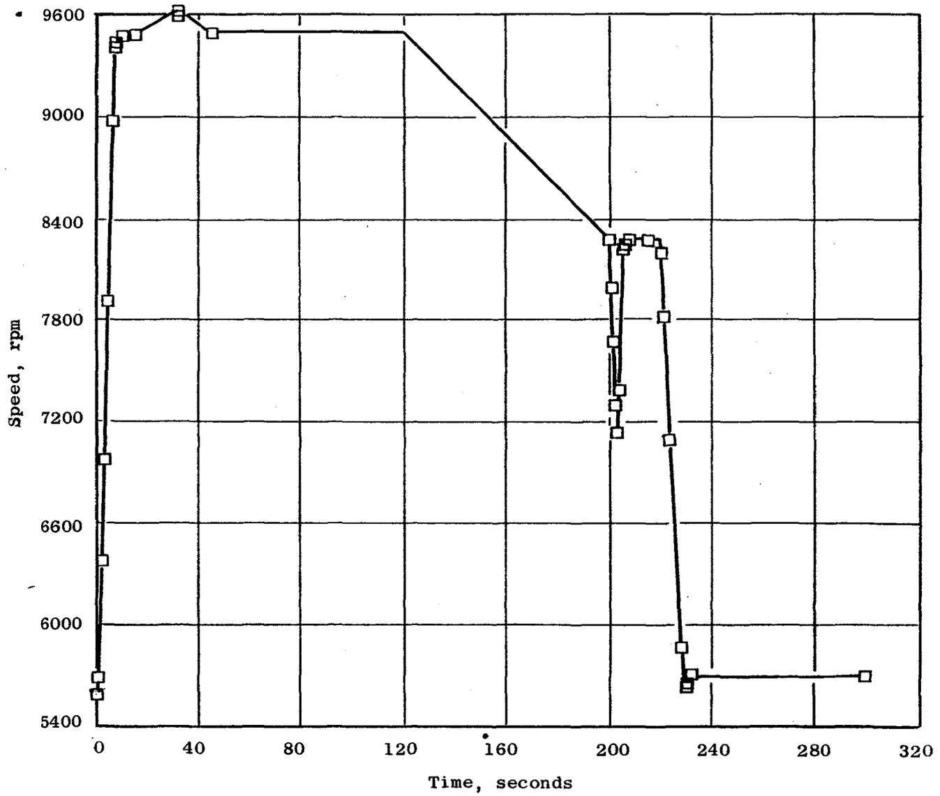
Figure 4.1-3. Mission Cycle Transient - Core Engine Speed.
