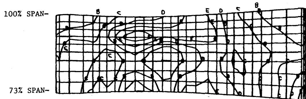
Figure 4.5-11. Blade Tip Model - Effective Stress Contour Plot -
