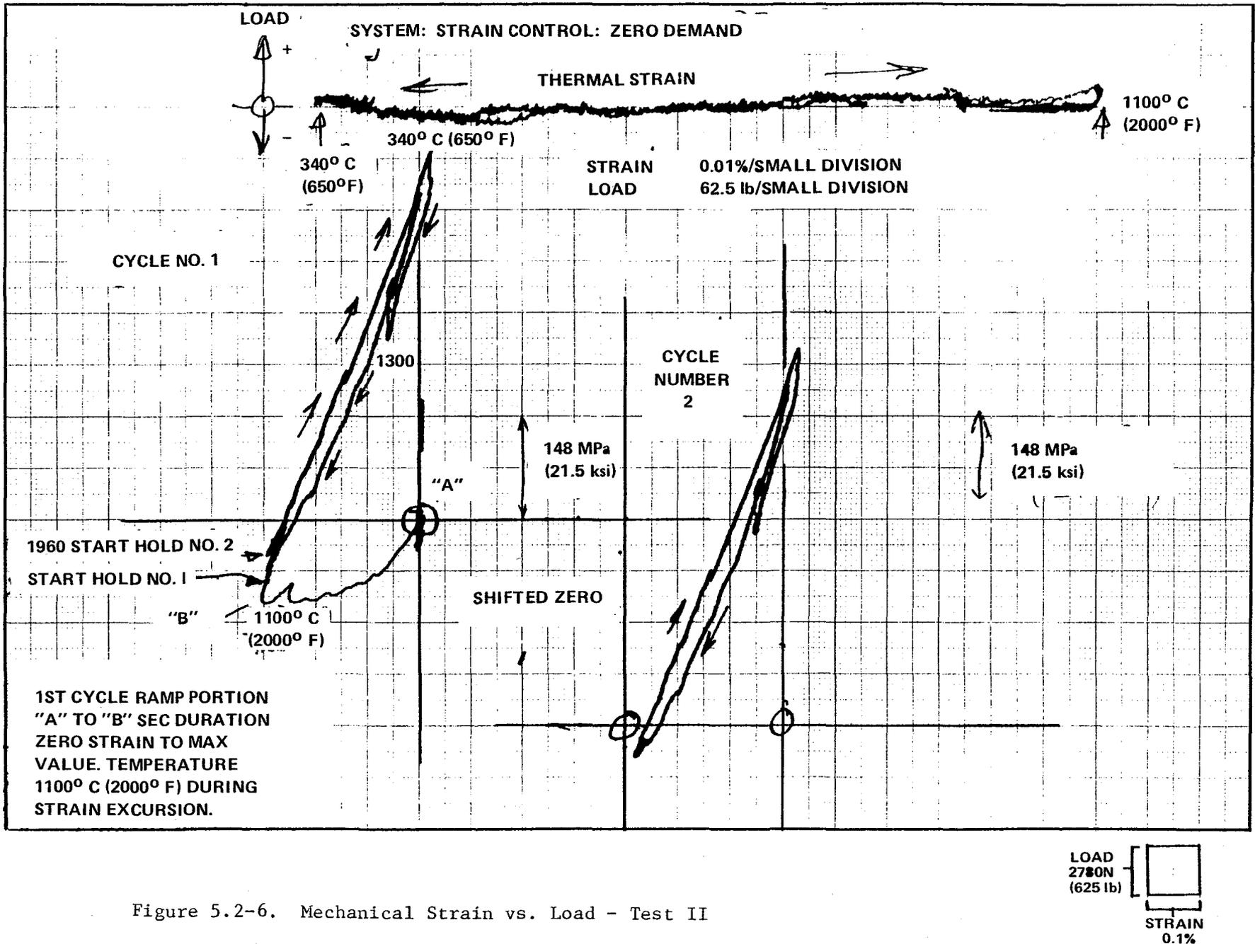
Figure 5.2-6. Mechanical Strain vs. Load - Test II
