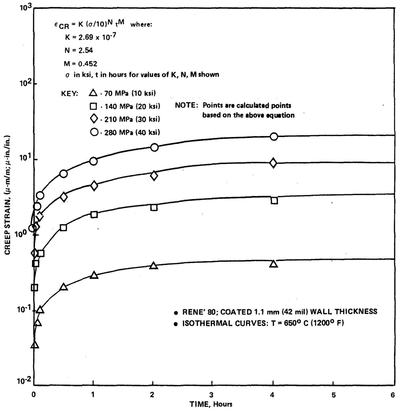
Figure 4.3-5. Creep Strain vs. Time for René 80.
