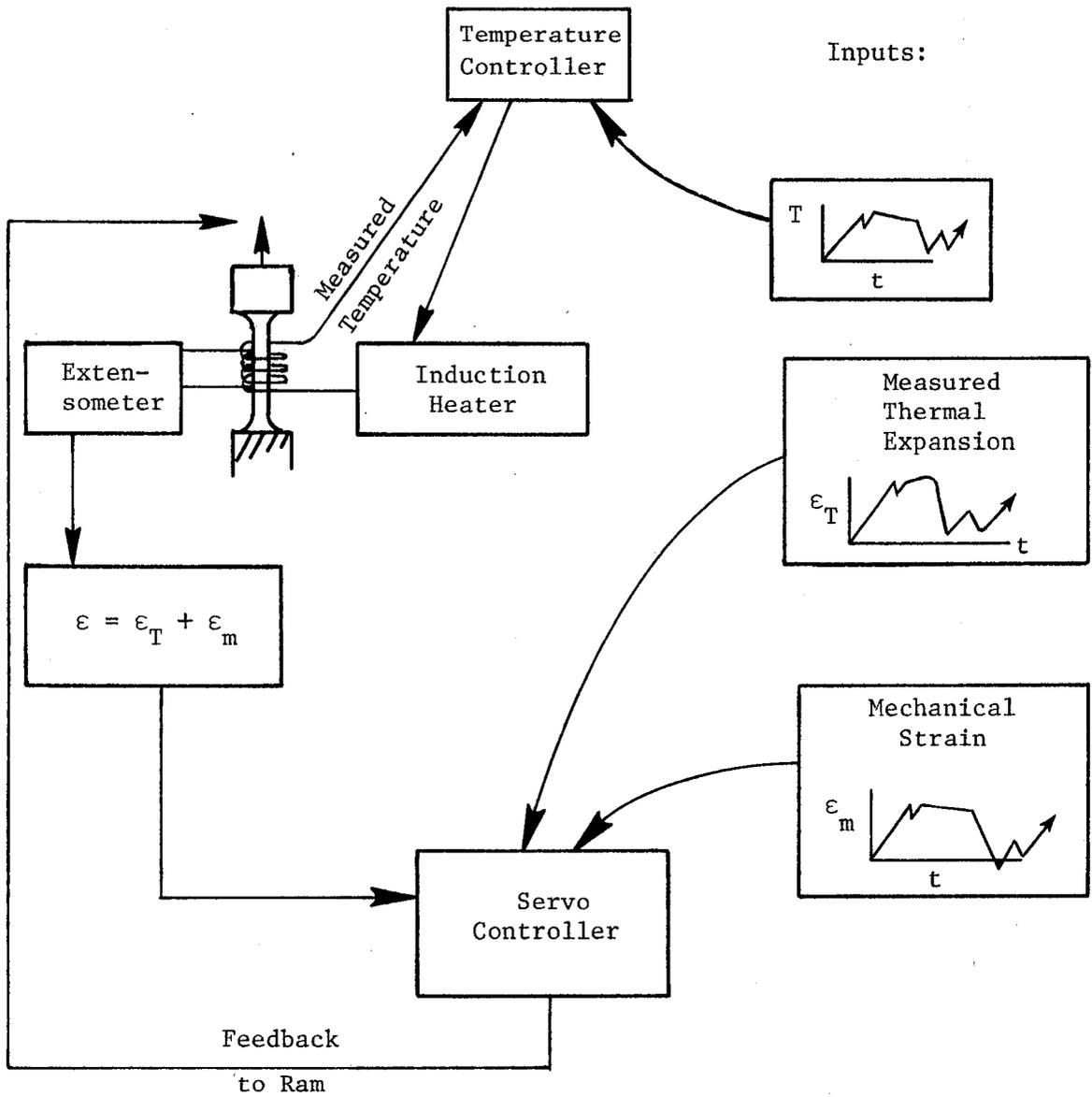
Figure 5.2-1. Schematic of TMF Setup.
