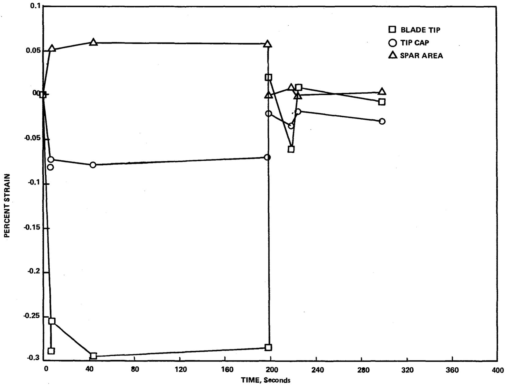
Figure 4.5-7. Principal Strain vs. Time for Critical Location (MASS Analysis).
