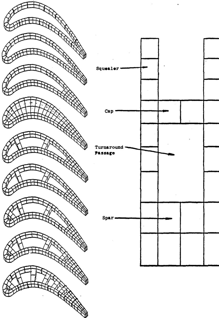
Figure 4.2-2. Details of 3-D Model of HPT Blade Tip.
