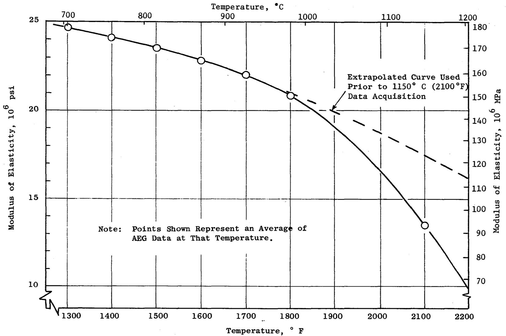
Figure 4.3-1. Elastic Modulus vs. Temperature for René 80.
