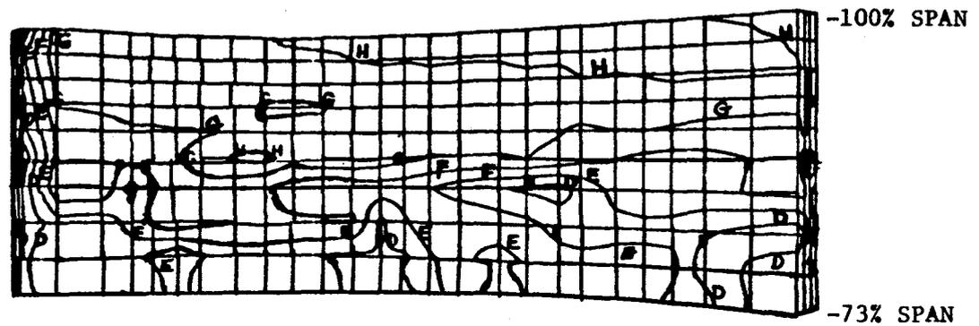
Figure 4.5-9. Blade Tip Model - Temperature Contour Plot - Pressure-Side Face.
