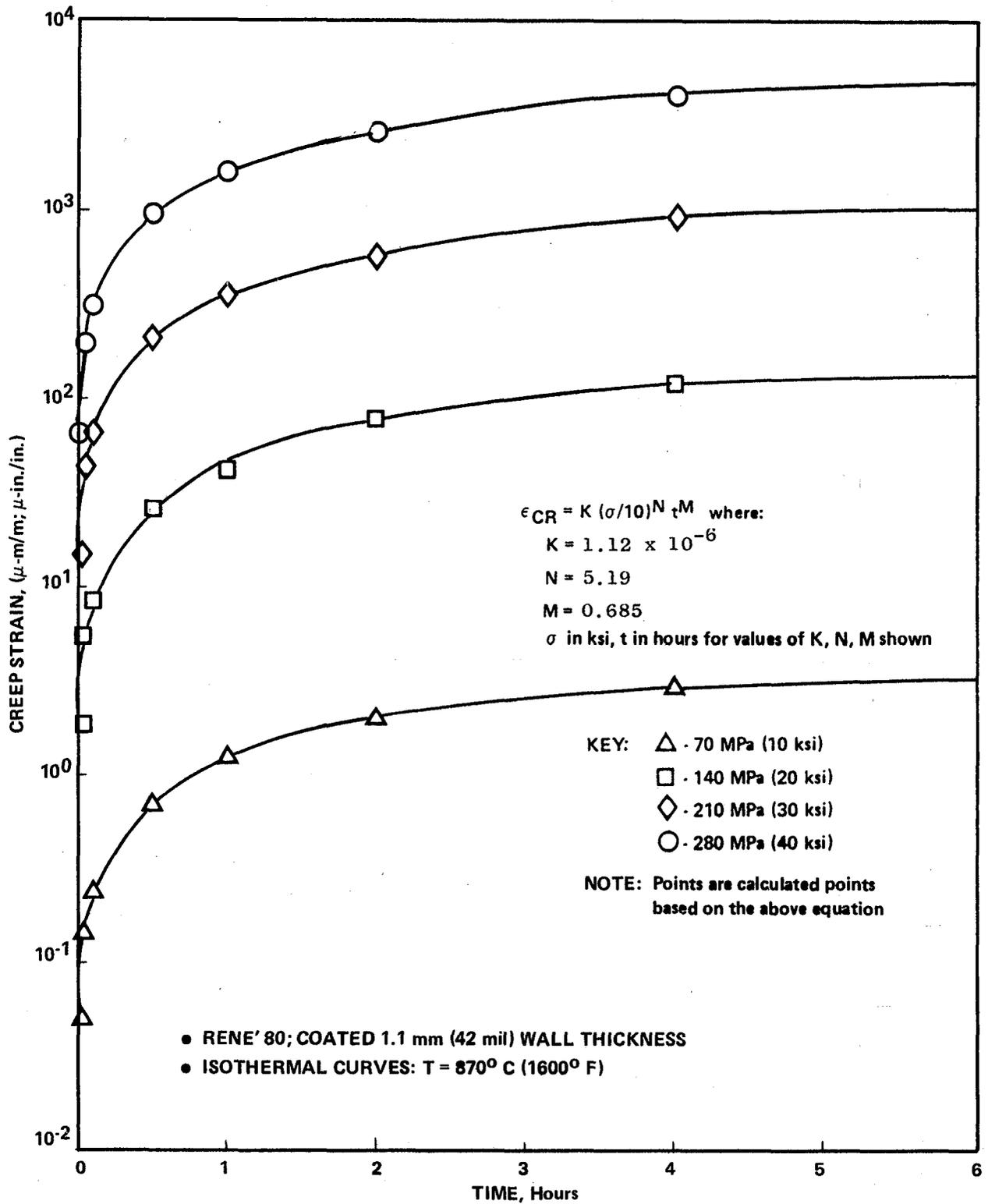
Figure 4.3-6. Creep Strain vs. Time for René 80.
