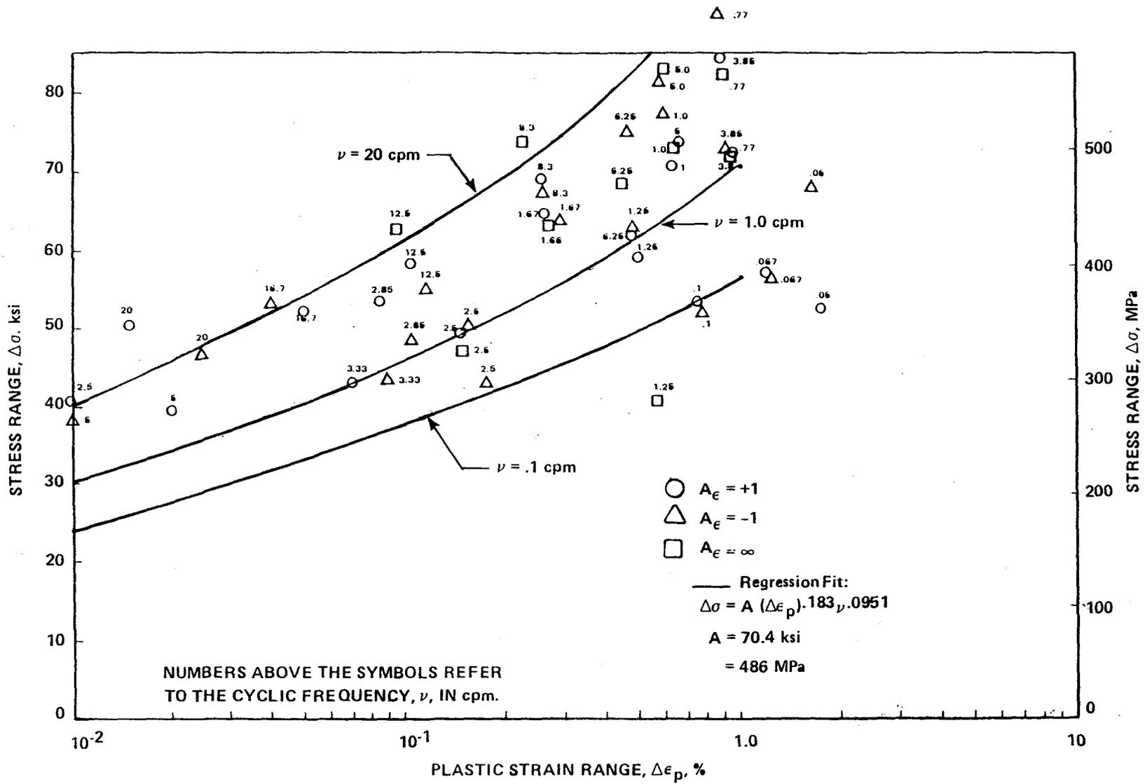
Figure 5.3-2. René 80 980° C (1800° F) FM Cyclic Stress-Strain Curve Fit.
