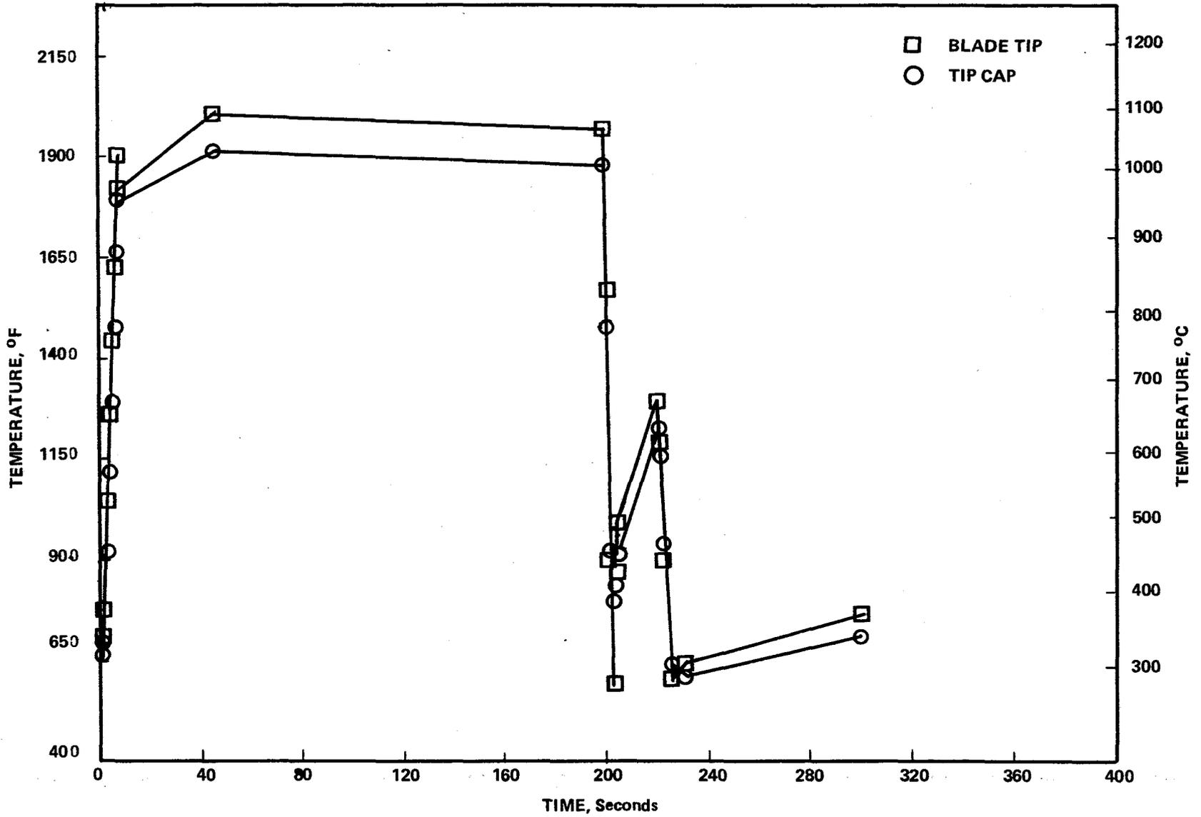
Figure 4.5-8. Blade Metal Temperature vs. Time for Critical Location.
