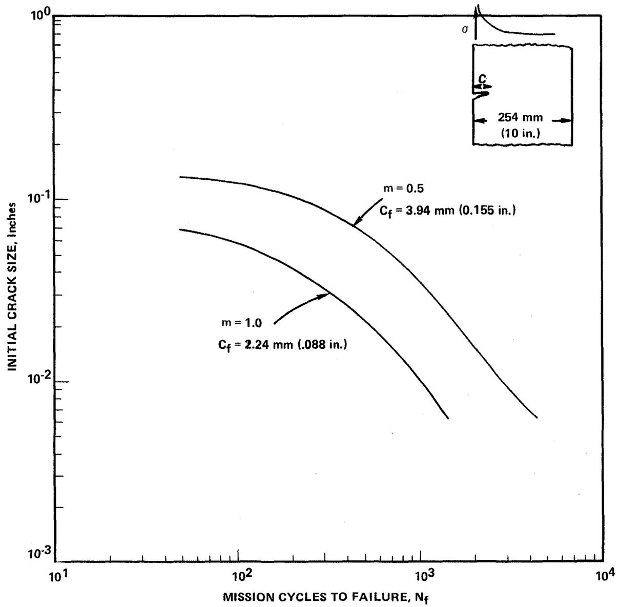
Figure 5.3-13. Results of the Crack Growth Analyses.
