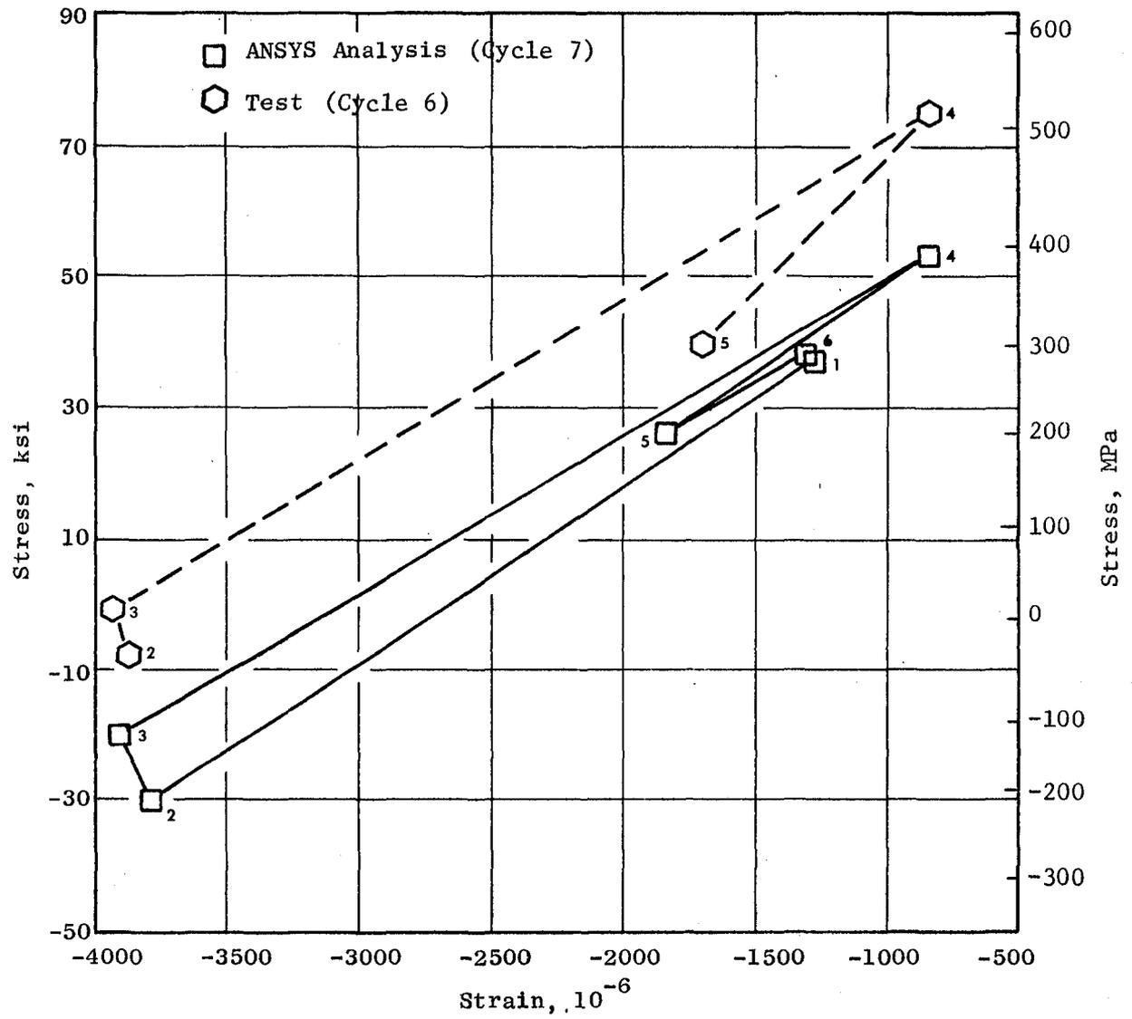
Figure 4.6-19. Stress Versus Strain - Inelastic Analysis Profile.
