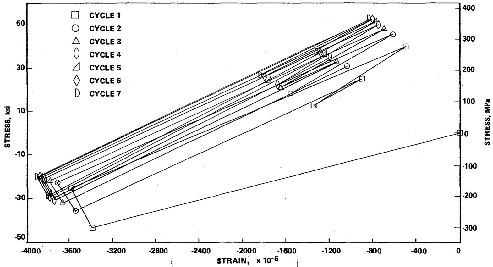
Figure 4.6-5. ANSYS Inelastic Analysis Results - Seven Cycles.
