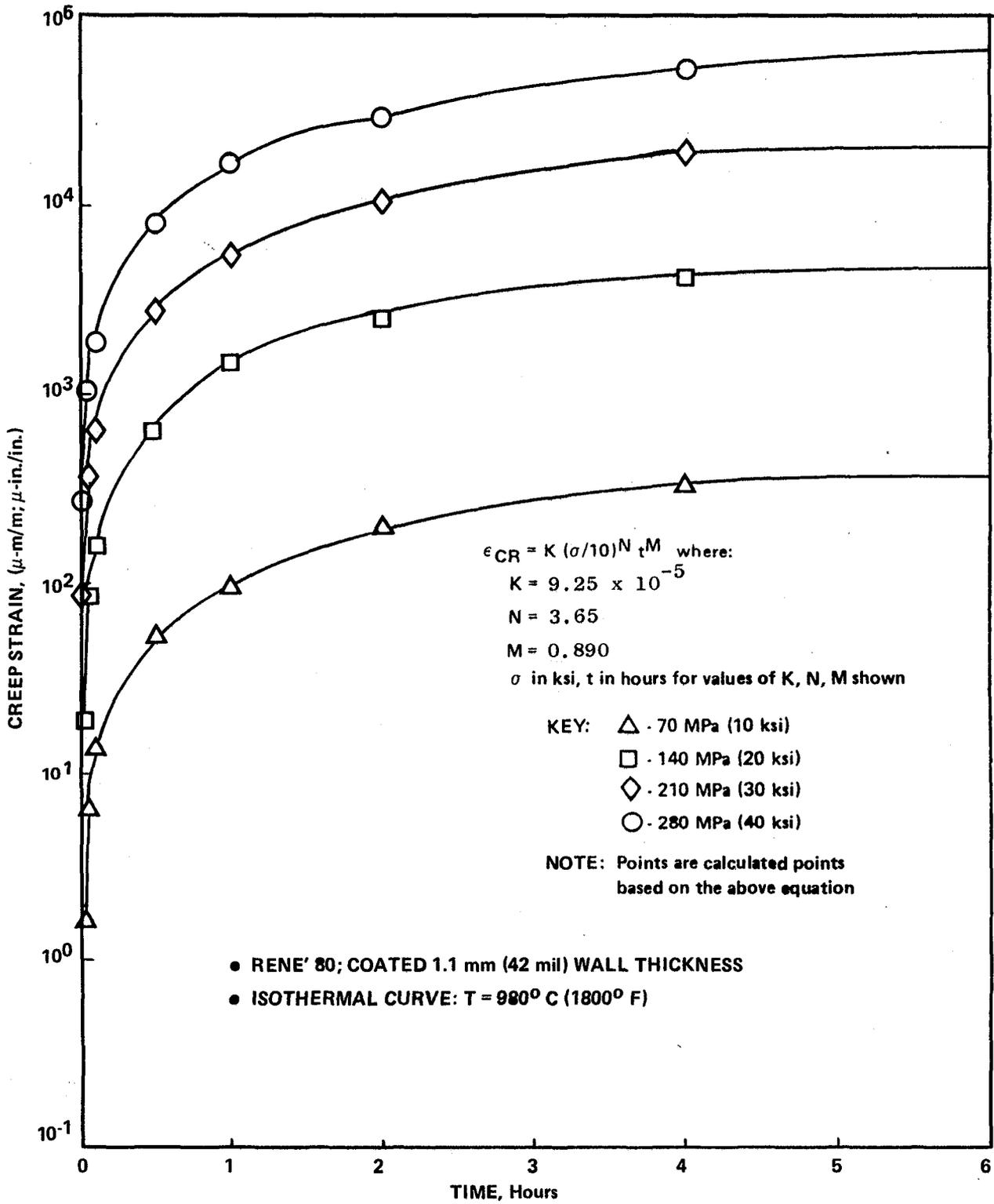
Figure 4.3-8. Creep Strain vs. Time for René 80.
