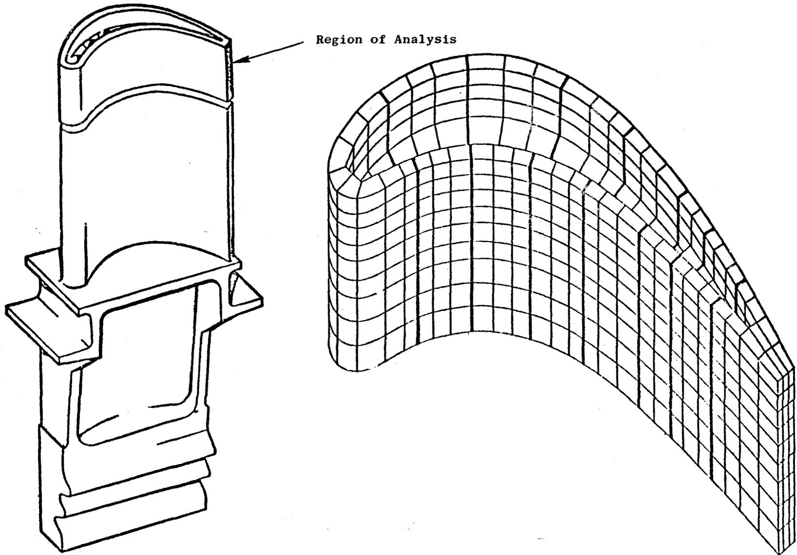
Figure 4.2-1. 3-D Model of HPT Blade Tip Region.
