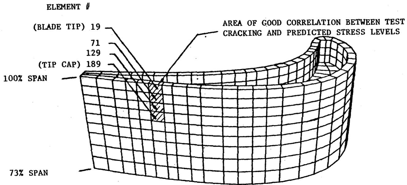
Figure 4.5-6. Blade Tip Location Chosen for Analysis.
