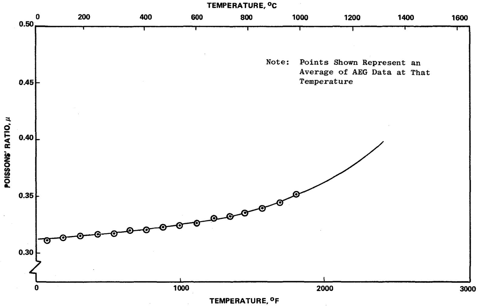
Figure 4.3-4. Poisson's Ratio vs. Temperature for René 80.
