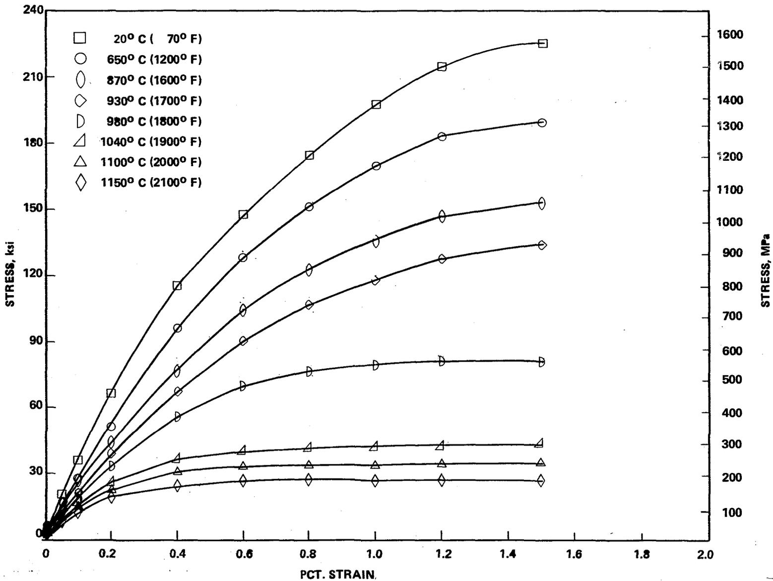
Figure 4.3-2. Cyclic Stress-Strain Curves for René 80.
