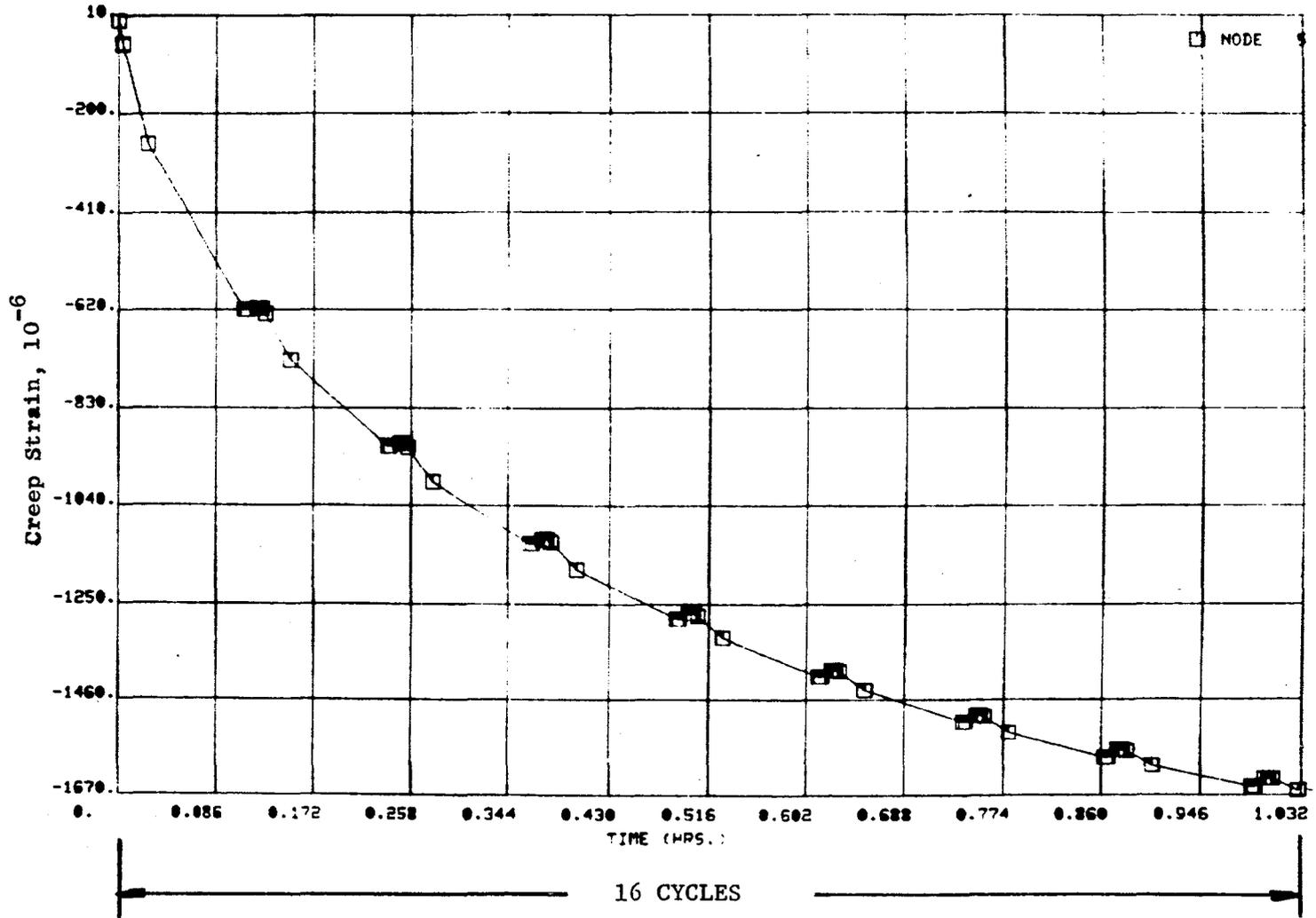
Figure 4.6-12. Cyanide Model Creep Strain vs. Time - Imposing Elastic Analysis Boundary Conditions.
