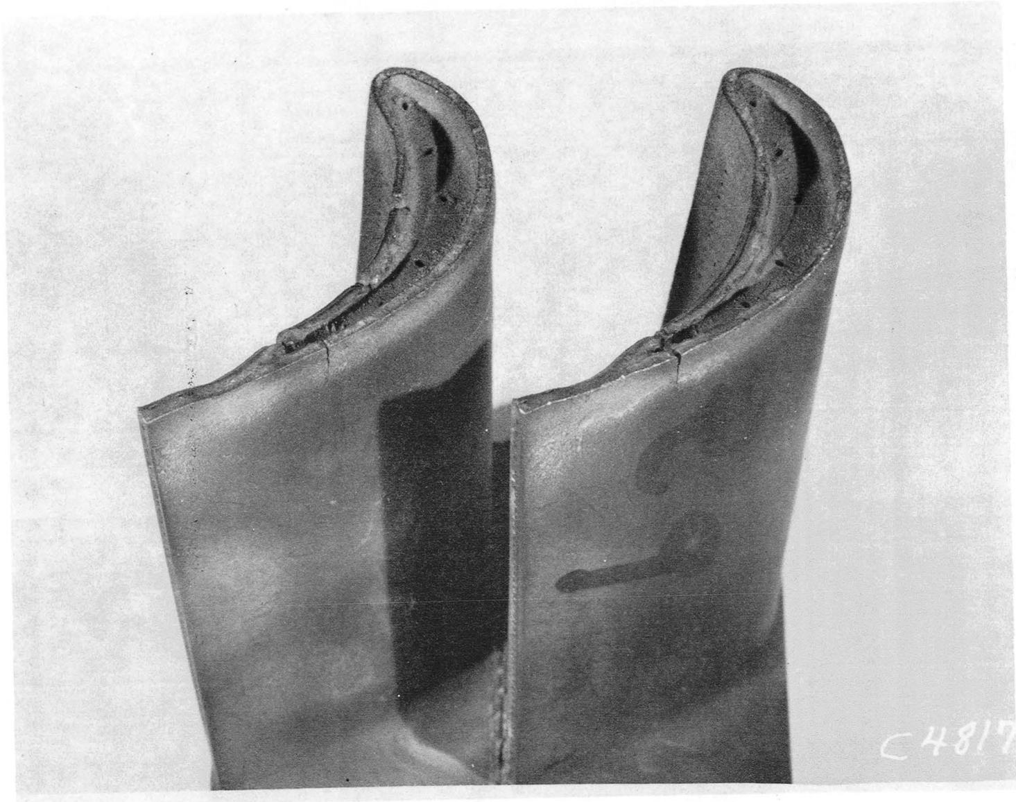
Figure 3.1-2. Typical Turbine Blade Tip Cracking - Example 1.
