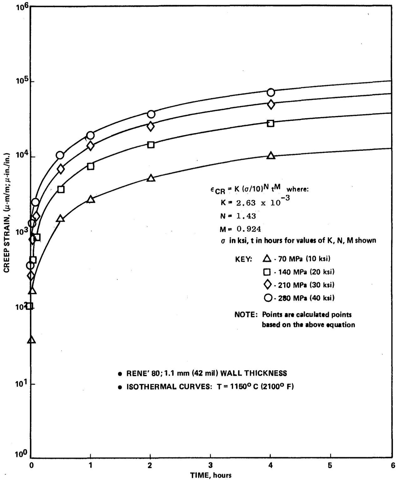
Figure 4.3-11. Creep Strain vs. Time for René 80.
