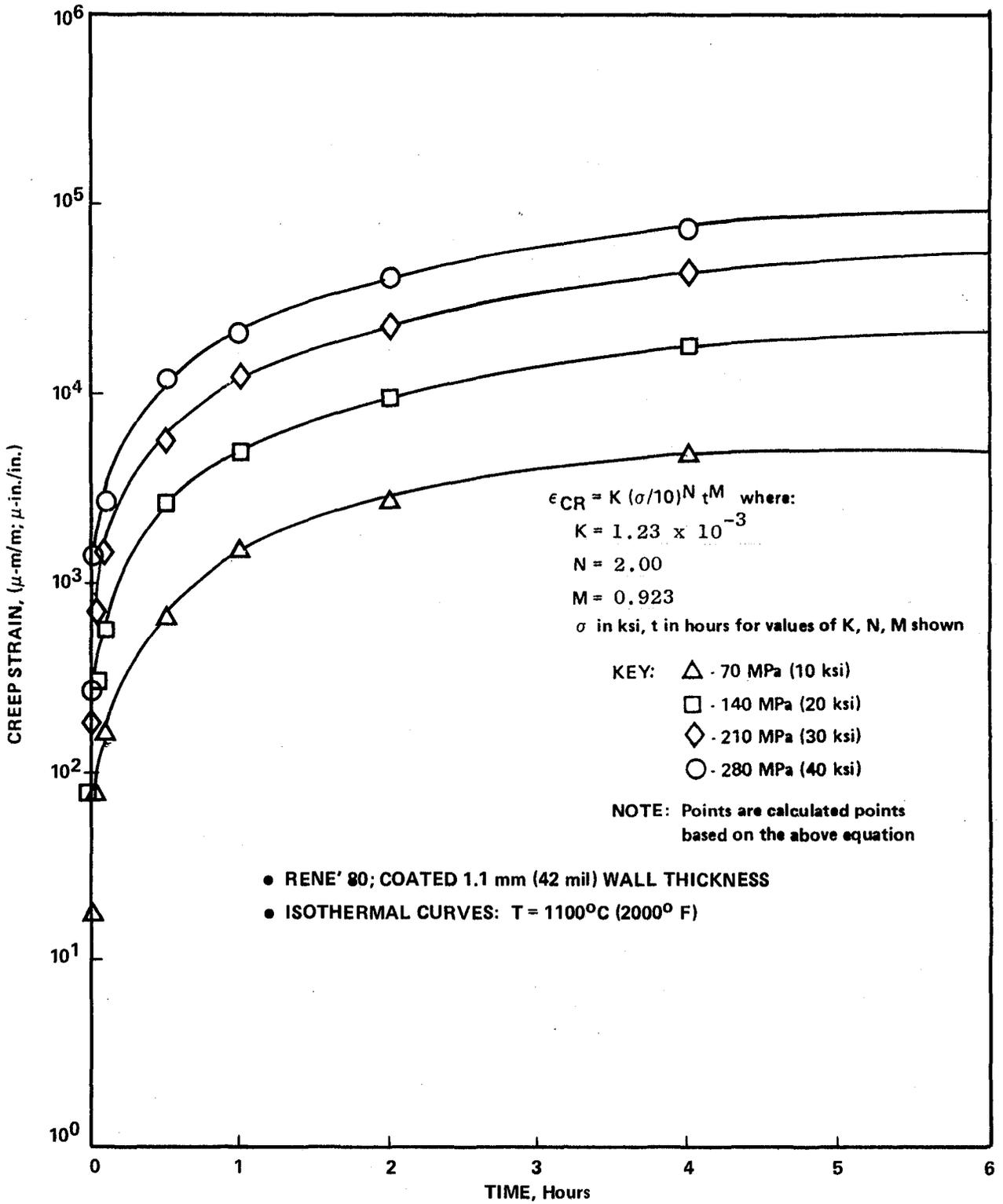
Figure 4.3-10. Creep Strain vs. Time for René 80.
