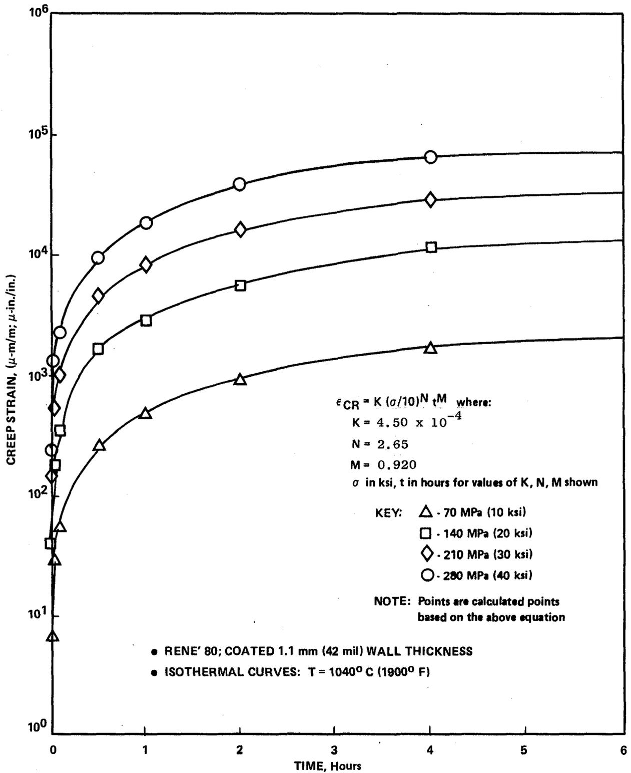
Figure 4.3-9. Creep Strain vs. Time for René 80.
