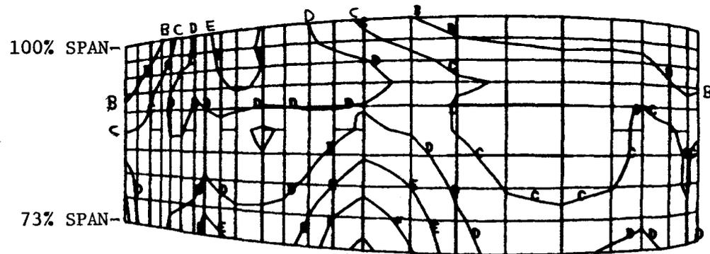
Figure 4.5-12. Blade Tip Model - Effective Stress Contour Plot -
