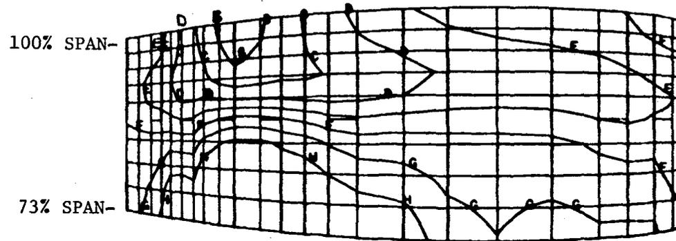
Figure 4.5-13. Blade Tip Model - Chordwise Stress Contour Plot -
