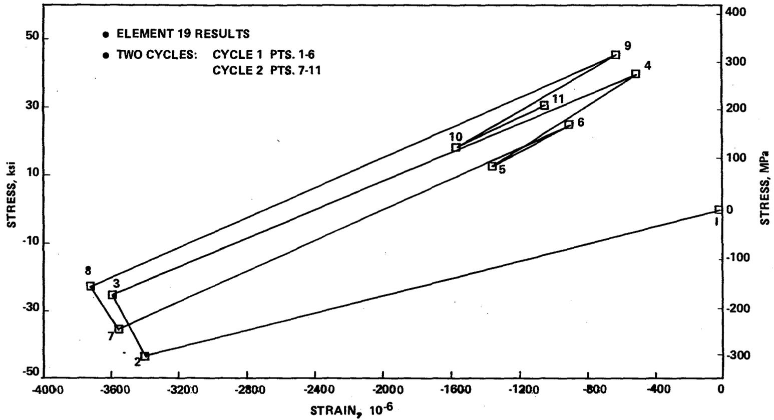
Figure 4.6-4. ANSYS Inelastic Analysis Results - Initial Two Cycles.
