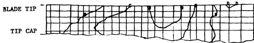
Figure 4.6-2. Blade Tip Model - Contour Plot of Principal Strains - Pressure-Side Face.
