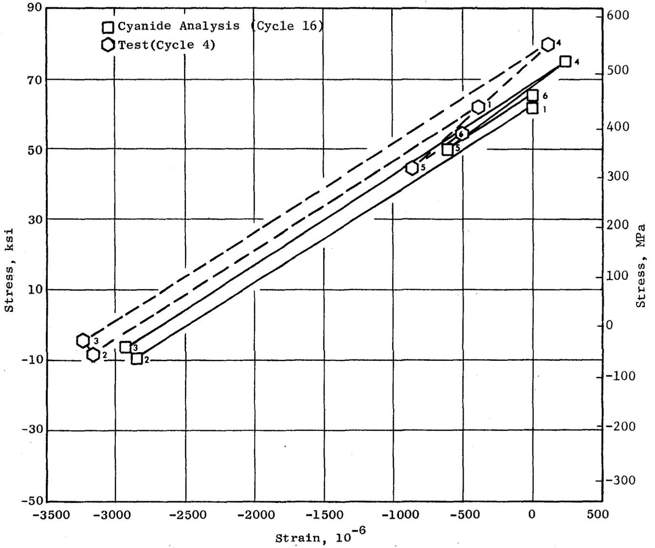
Figure 4.6-18. Stress Versus Strain - Elastic Analysis Profile.
