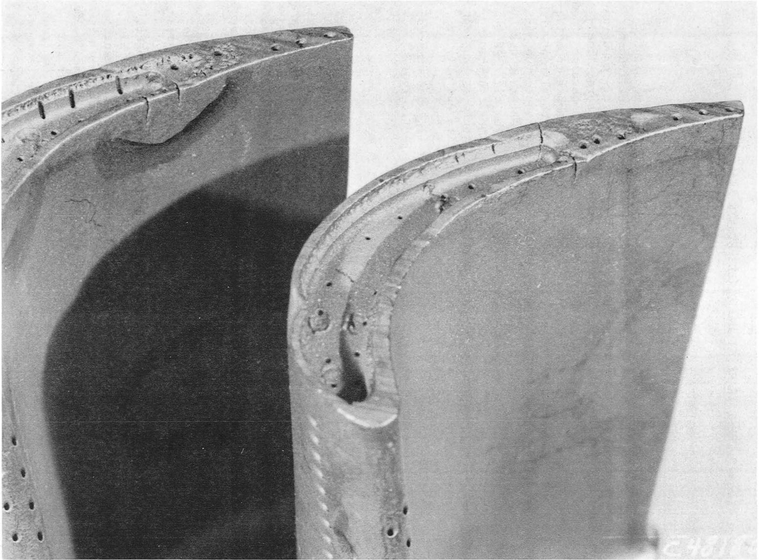
Figure 3.1-4. Typical Turbine Blade Tip Cracking - Example 3.
