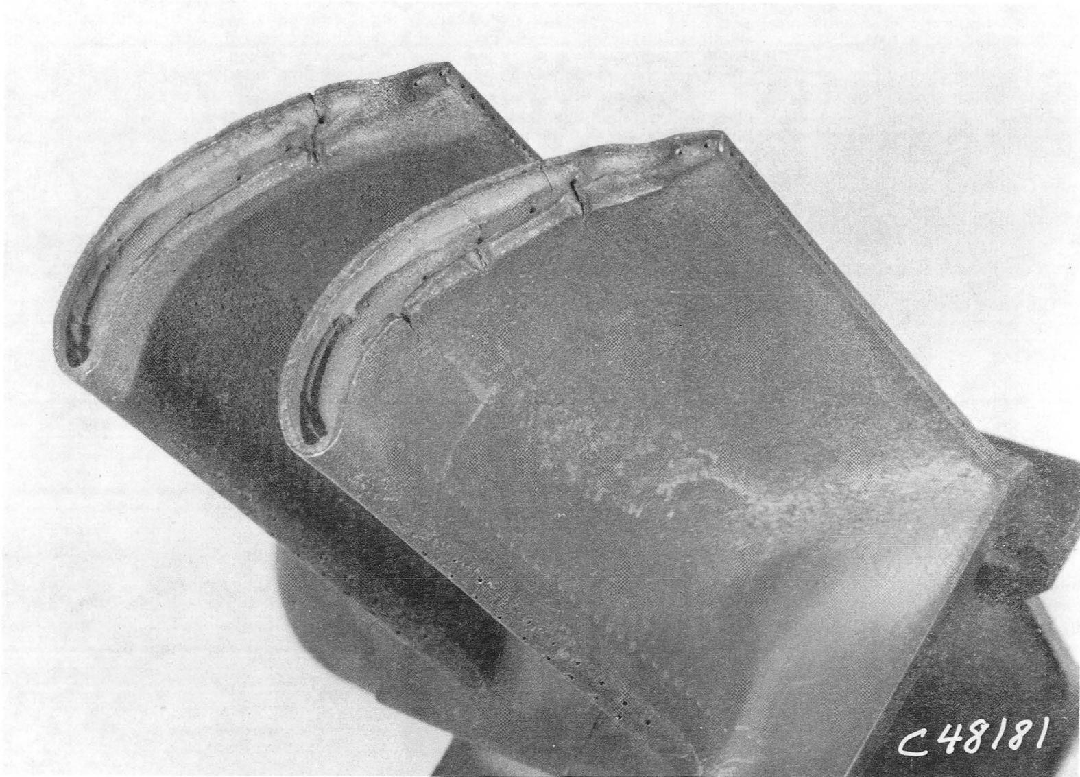
Figure 3.1-3. Typical Turbine Blade Tip Cracking - Example 2.
