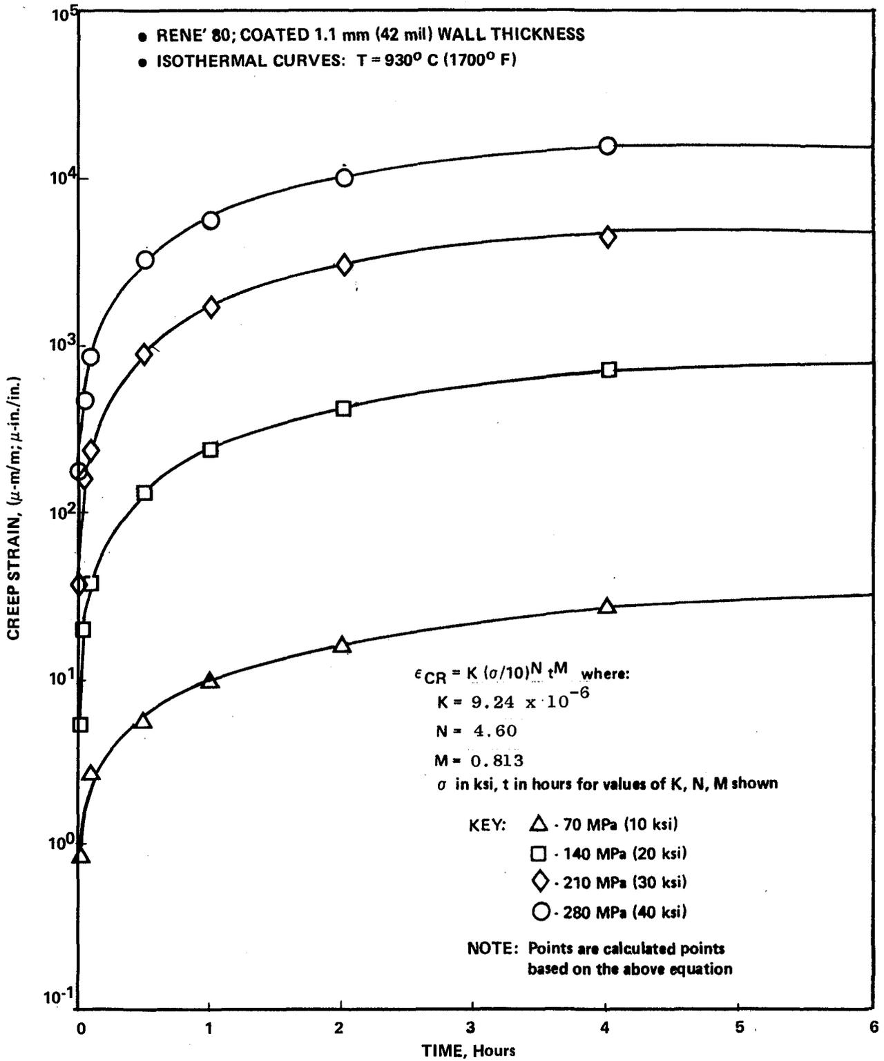
Figure 4.3-7. Creep Strain vs. Time for René 80.
