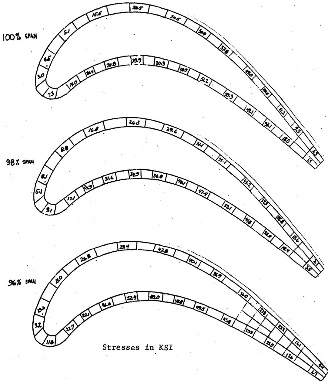
Figure 4.5-3. 3-D Elastic Stress Analysis - Squealer Tip Region - Chordwise Stresses.
