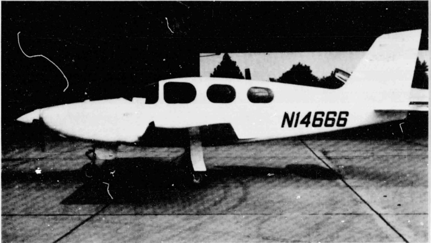
A laminar-flow-controlled wing applied to a general aviation aircraft.
