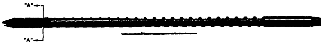
Figure 5-4. A Photograph of the -2 Screw Configuration Showing the Mixer Section in Place
