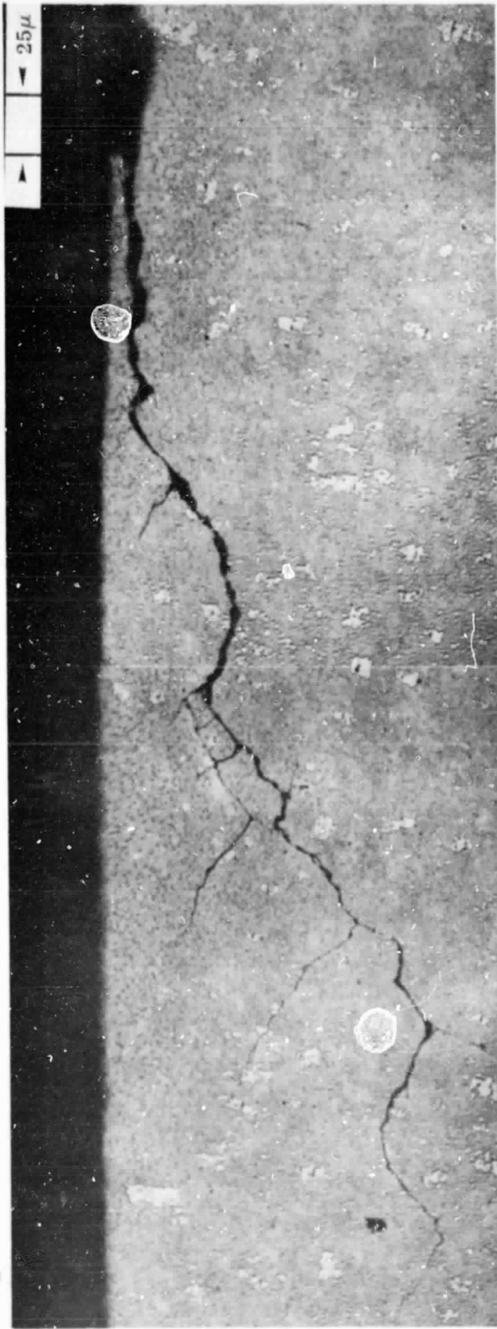
Figure 15. Shallow crack in HPOTP 9008 bearing ball from Engine 2004. Crack depth approximately 0.13 mm (0.005 in.) (area C in Figure 12).
