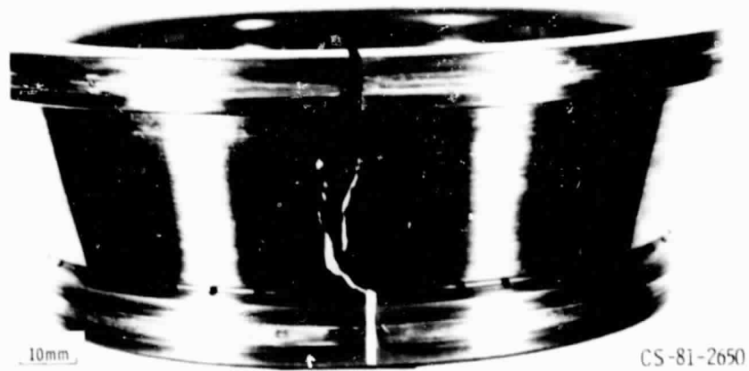
Figure 7. - Fractured cone of AISI M-50 bearing S/N 78-10 after 188 hours of operation at 18 500 rpm.
