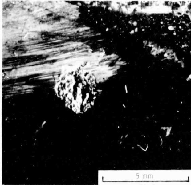
Figure 9. - Fatigue spall on cone raceway of CBS-1000M bearing S/N 76-17 after 135 hours of operation at 18 500 rpm.
