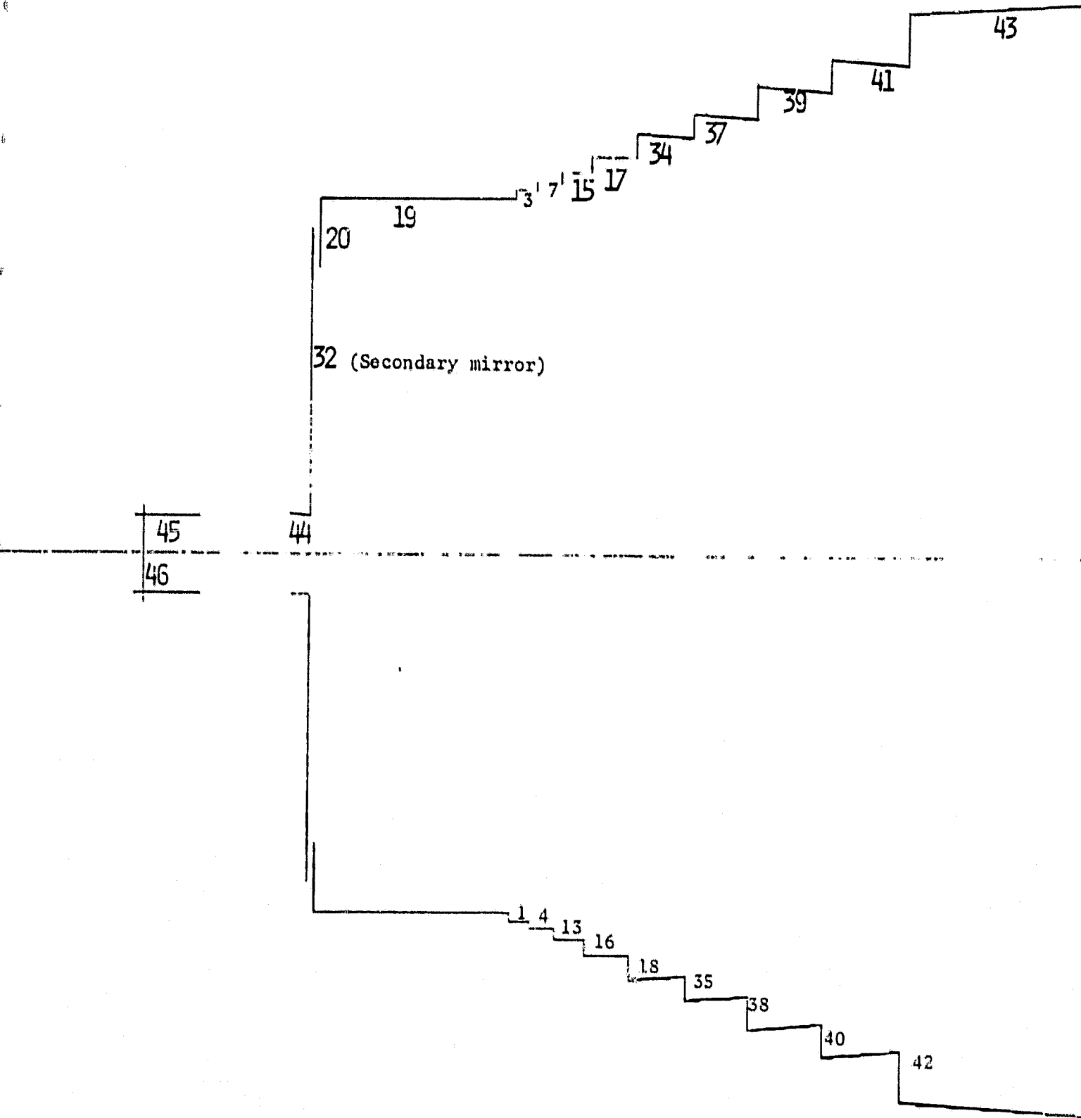
Figure 2. Details of the secondary baffle.
