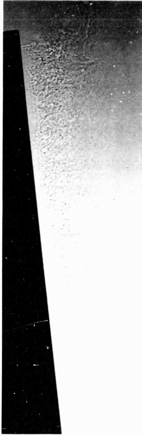
Figure 6. Shadowgraph Showing Entrained Flow of a Jet. Velocity at Nozzle Exit = 152 m/s.
