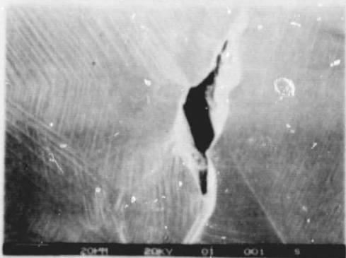
e) Stereoscan, x 400 (internal crack)
