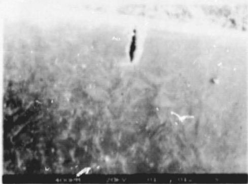
a) Stereoscan, x 20 (edge crack)
