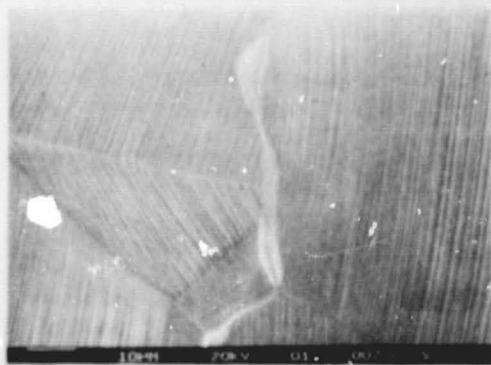
g) Stereoscan, x 800 (bond line)
