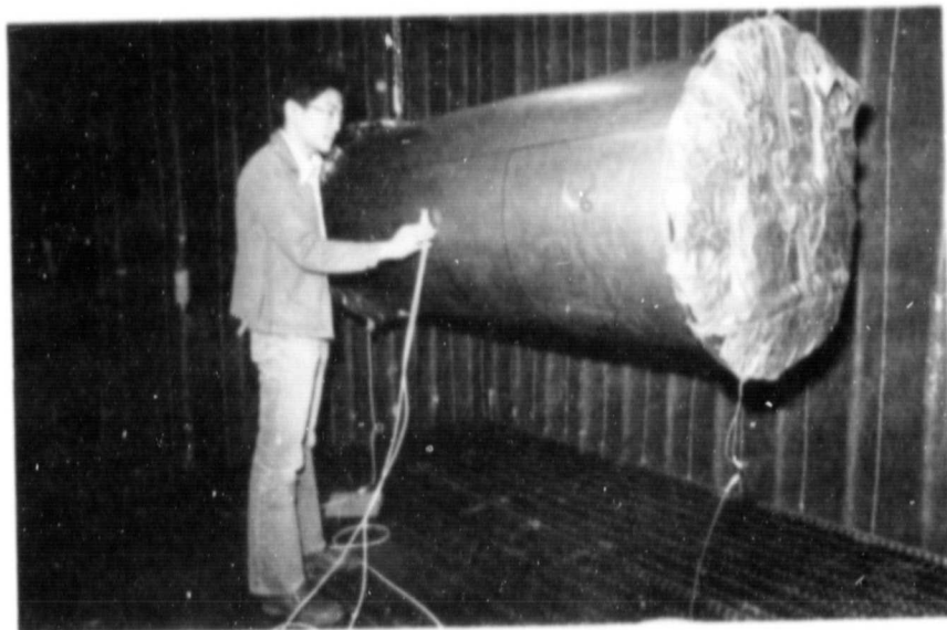
Fig. 3.6a Acoustic Intensity Measurement on the Cylindrical Shell.
