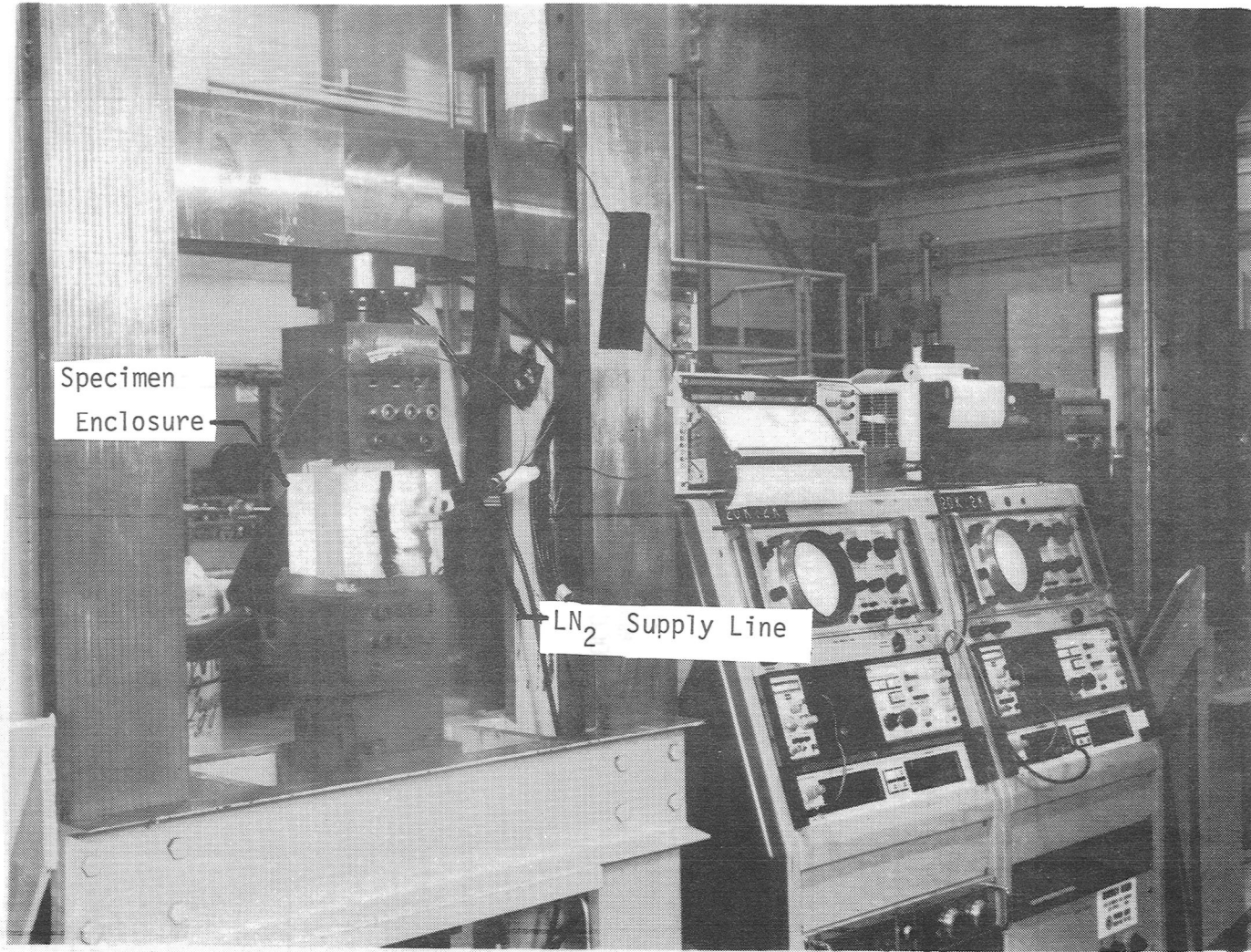
Figure 17.- Fatigue test setup for the cold temperature tests.
