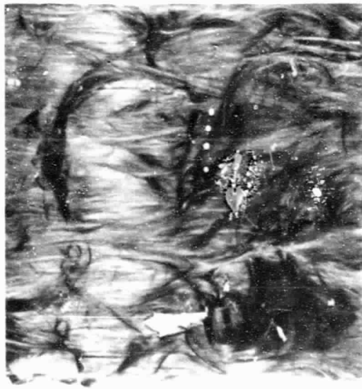
Figure 20: Unfilled (Control) Specimen After OSU Exposure ( 10W/cm^2 )
