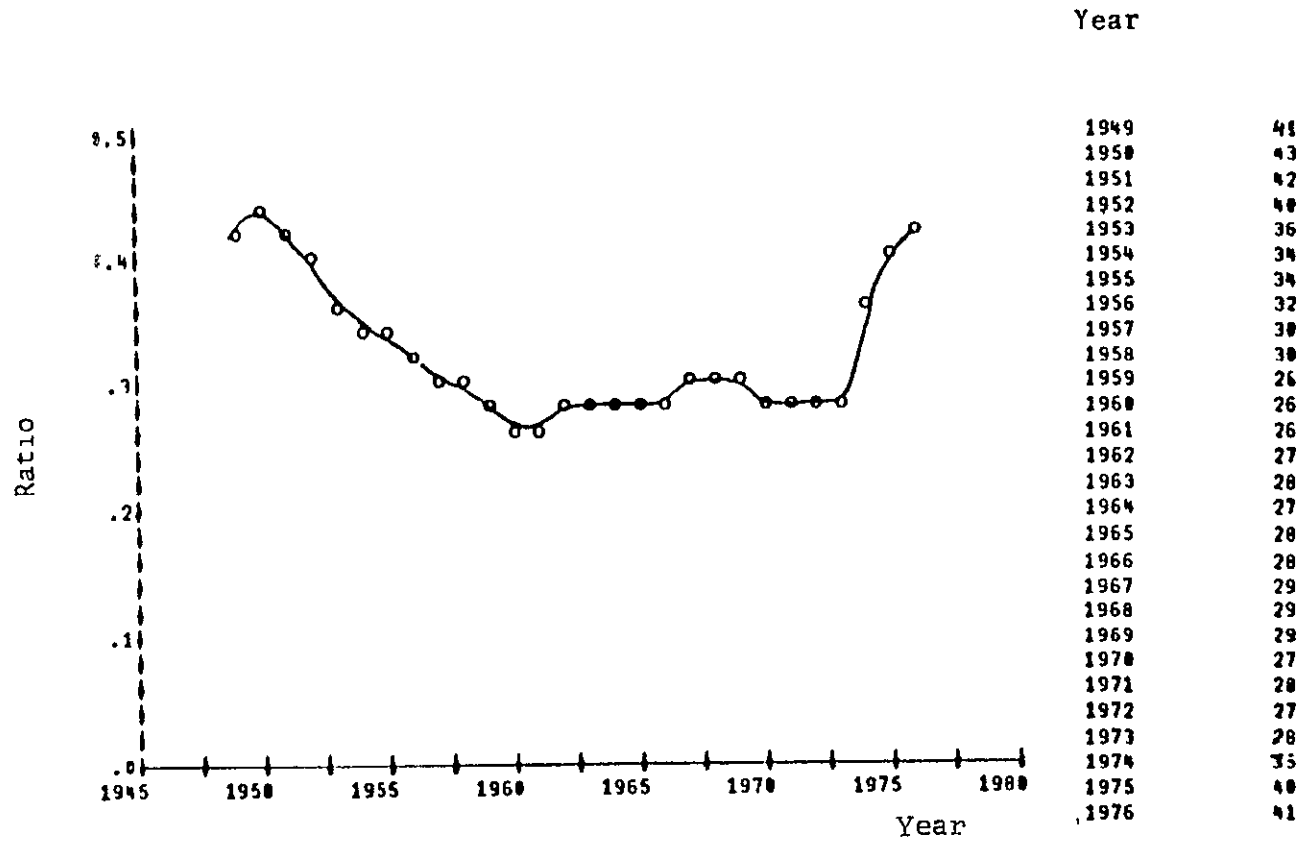
Figure IV - 32 Ratio of Fuel Cost to Direct Operating Costs, Certificated Air Carriers
