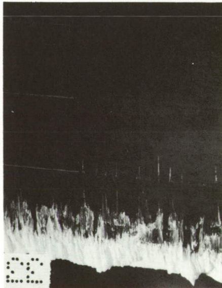
(a) Boot A after 6 minutes in icing.
