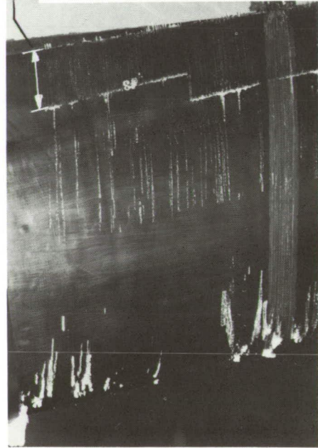
(c) Boot C after 22 minutes in icing.
