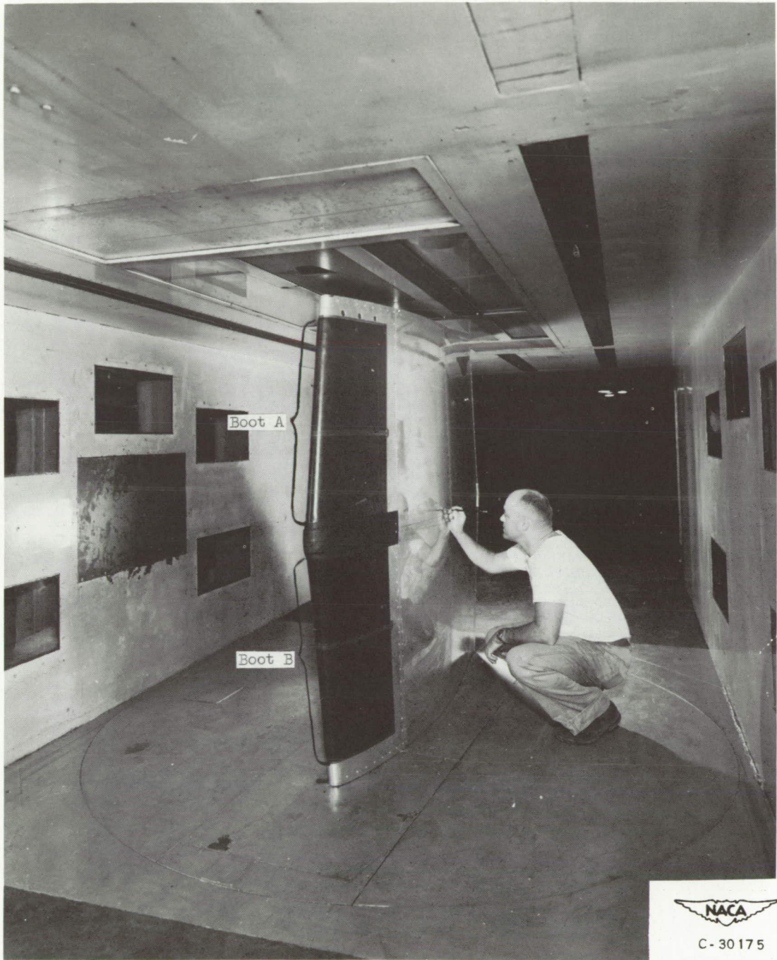
Figure 1. - Installation of airfoil model in test section of icing research tunnel.
