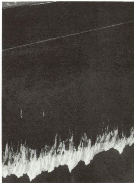
(b) Boot B after 6 minutes in icing.
