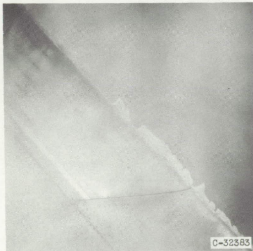
Upper surface. Icing time, 13\frac{1}{2} minutes; section drag coefficient, 0.0358.
