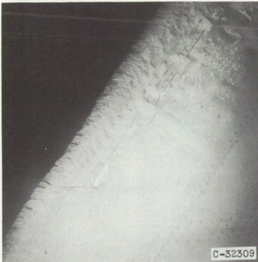
Lower surface. Icing time, 10\frac{1}{2} minutes; section drag coefficient, 0.0350.
