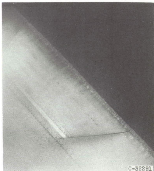
Upper surface. Icing time, 5 minutes; section drag coefficient, 0.0199.
