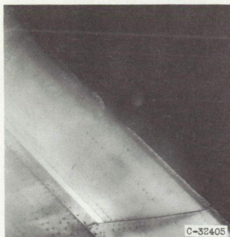
Upper surface. Icing time, 39\frac{1}{2} minutes; section drag coefficient, 0.0136; slatted airfoil; heat-on period, 20 seconds; heat-off period, 460 seconds.
