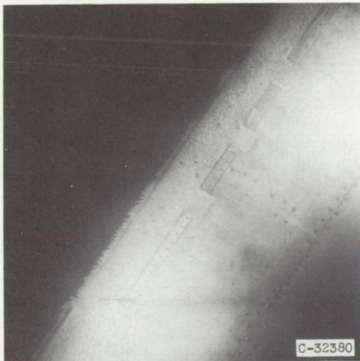
Lower surface. Icing time, 4 minutes; section drag coefficient, 0.0192.
