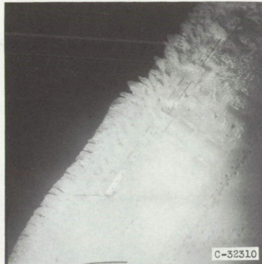
Lower surface. Icing time, 11 minutes; section drag coefficient, 0.0360.
