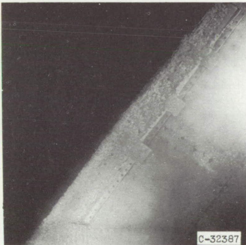
Lower surface. Icing time, 10 minutes; section drag coefficient, 0.0153.
