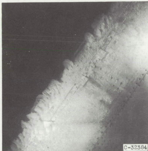
Lower surface. Icing time, 16\frac{1}{2} minutes; section drag coefficient, 0.0461.
