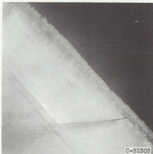
Upper surface. Icing time, 10\frac{1}{2} minutes; section drag coefficient, 0.0321.
