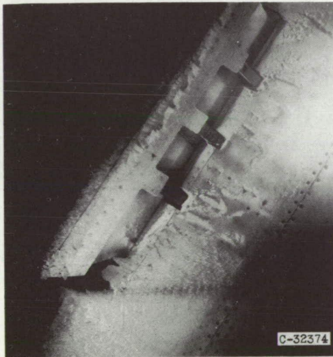
Lower surface. Icing time, 10 minutes; section drag coefficient, 0.0602.
