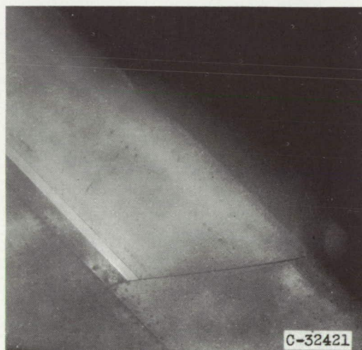
Upper surface. Icing time, 16 minutes; section drag coefficient, 0.0130; before ice removal; slatted airfoil.
