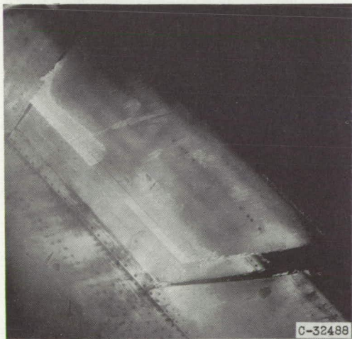
Upper surface. Icing time, 36\frac{1}{2} minutes; section drag coefficient, 0.0394; before ice removal.
