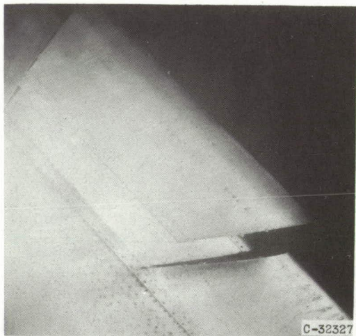
Upper surface. Icing time, 11\frac{1}{2} minutes; section drag coefficient, 0.0440; before ice removal.
