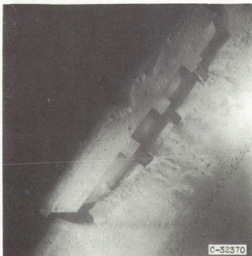
Lower surface. Icing time, 10\frac{1}{2} minutes; section drag coefficient, 0.0490.
