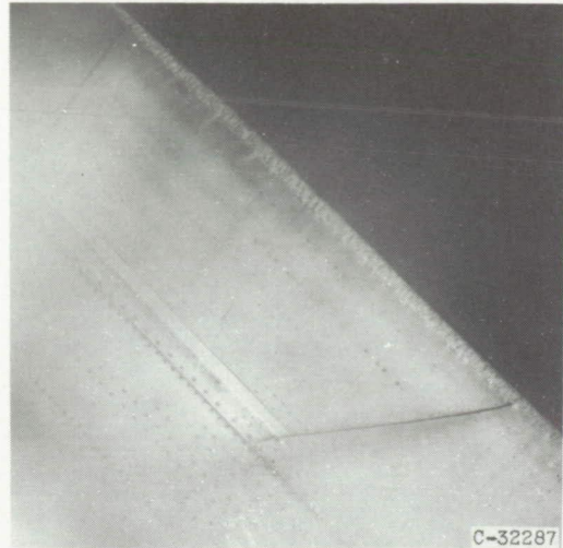
Upper surface. Icing time, 5\frac{1}{2} minutes; section drag coefficient, 0.0177.
