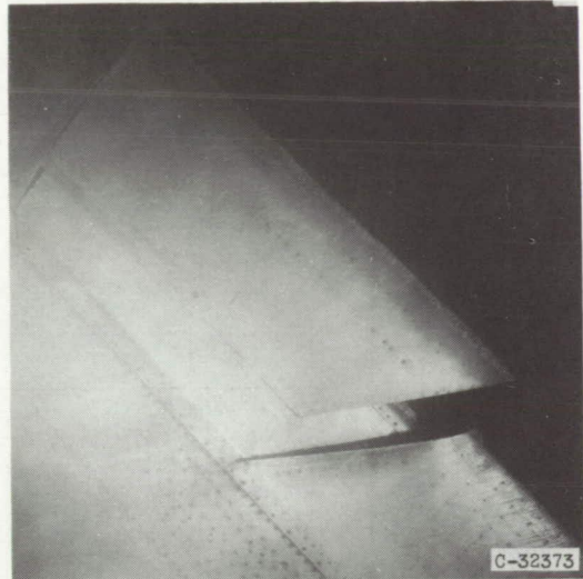
Upper surface. Icing time, 4 minutes; section drag coefficient, 0.0450.
