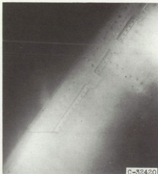
Lower surface. Icing time, 12\frac{1}{2} minutes; section drag coefficient, 0.0122; after ice removal; standard airfoil.
