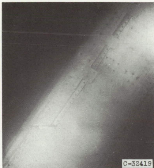
Lower surface. Icing time, 12 minutes; section drag coefficient, 0.0138; before ice removal; standard airfoil.
