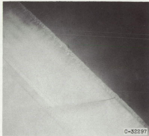
Upper surface. Icing time, 5 minutes; section drag coefficient, 0.0188.
