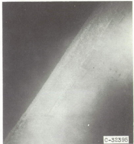
Lower surface. Icing time, 11 minutes; section drag coefficient, 0.0134.
