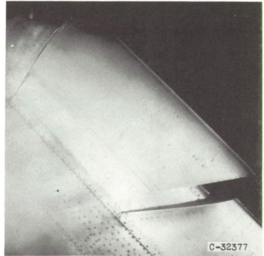
Upper surface. Icing time, 5 minutes; section drag coefficient, 0.0317.
