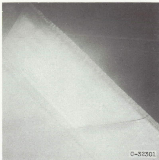
Upper surface. Icing time, 4\frac{1}{2} minutes; section drag coefficient, 0.0188.
