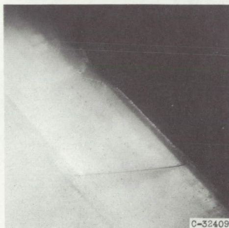
Upper surface. Icing time, 54\frac{1}{2} minutes; section drag coefficient, 0.0145; slatted airfoil; heat-on period, 10 seconds; heat-off period, 470 seconds.
