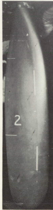
(a) 25-percent partitioned blade: indicated tunnel air temperature, 23° F; heating rate, 7000 Btu per hour per blade.
