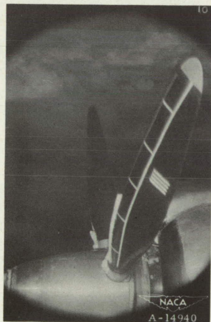
Figure 20.- Ice formation of encounter 3. Camber face. Peak efficiency loss, 4 percent at \beta_0 = 25.8^\circ ; 6 percent at \beta_0 = 31.8^\circ .
