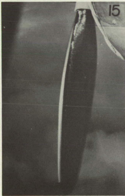
Figure 28.— Ice formation of encounter 10. Thrust face. Efficiency loss, 0 percent.
