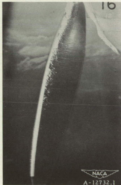
Figure 30.— Ice formation of encounter 11. Thrust face. Efficiency loss, 0 percent.
