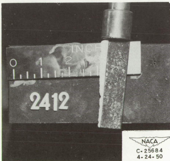
(b) Configuration E; round-wire screen; icing period, 11 minutes; initial mass flow per unit area, 24.5 pounds per second per square foot.
