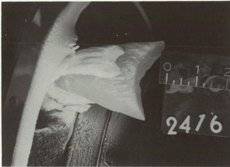
(a) Configuration A; no screen; icing period, 15 minutes; initial mass flow per unit area, 28.4 pounds per second per square foot.
