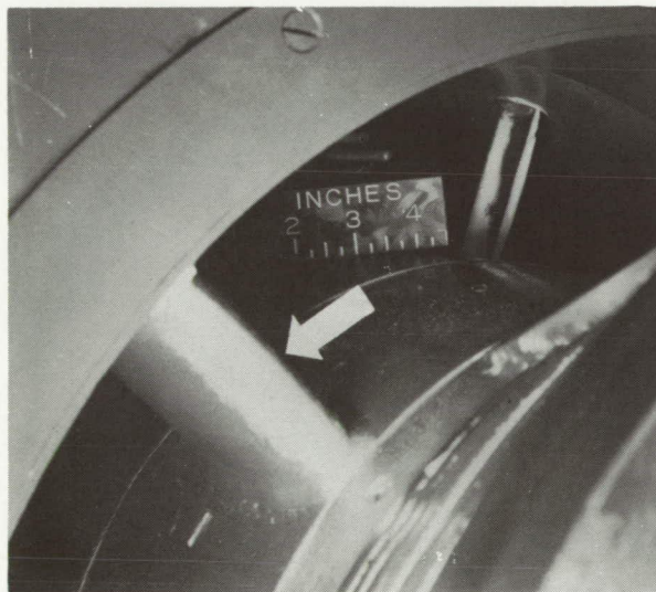
(b) Configuration C; streamlined-wire screen; icing period, 10 minutes; initial mass flow per unit area, 27.2 pounds per second per square foot.
