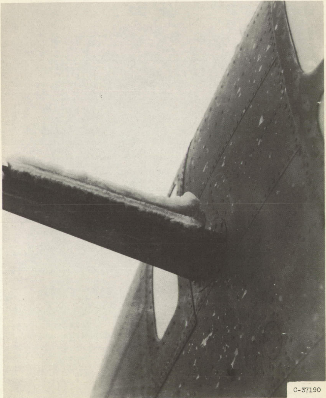
Figure 1. - Ice formation on pitot mast on B-24 aircraft after flight through supercooled clouds.
